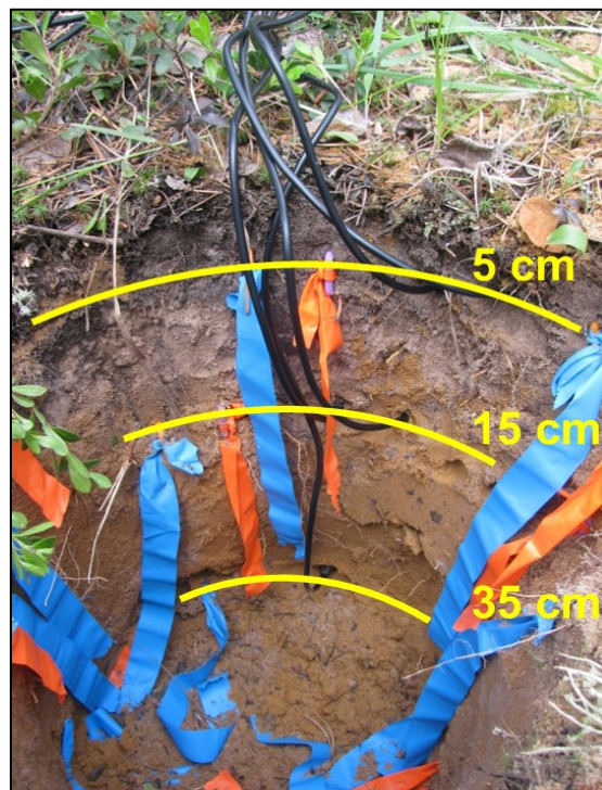
Figure 6.6 – Pit setup for PRS™ probes and temperature and moisture sensors in the Aurora Soil Capping Study.
