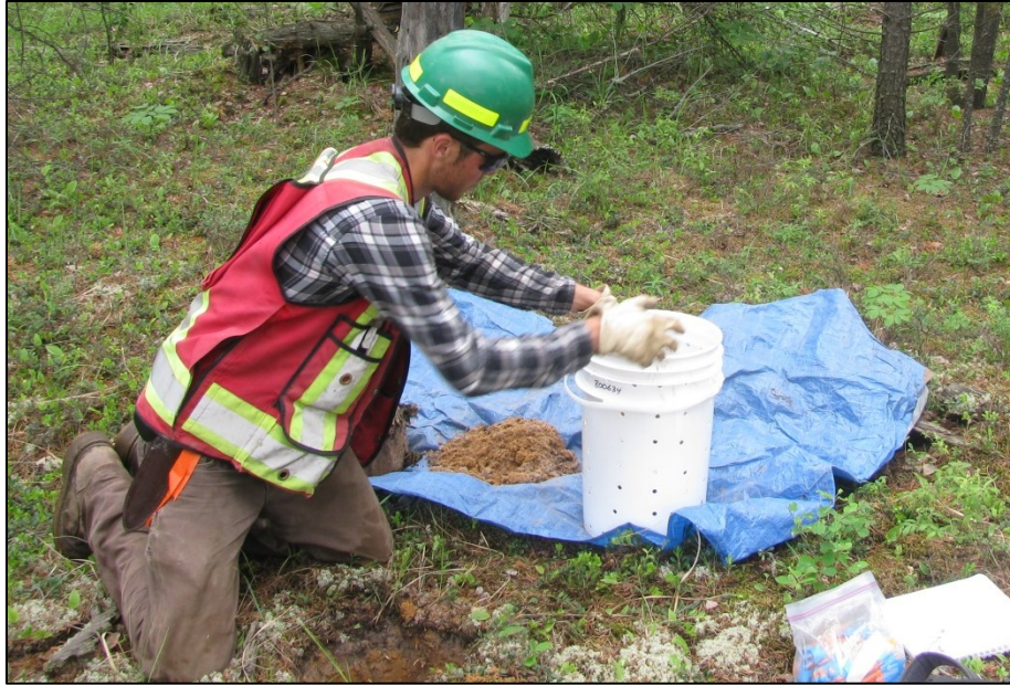
Figure 6.5 – Perforated 20 liter polyethylene pails for backfilling sampling pits that were instrumented with ionic exchange membranes, temperature and moisture sensors in the Aurora Soil Capping Study.
