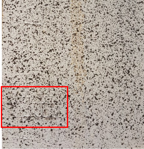
Figure 4.17: Yielding of the Non-Bolted Flange at 75% Axial Load
