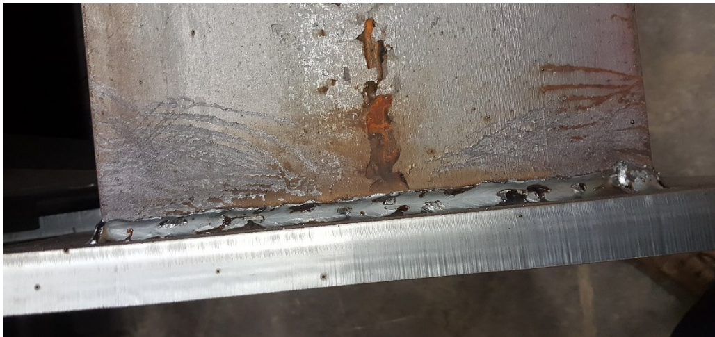
Figure 4.18: Yielding of the Bolted Flange at the Ends of the Test Specimen
