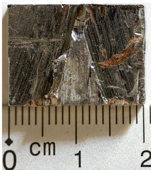
Figure 4.22: Crack surface of sample X70-X. The triangular, lighter grey area is the opened crack.
