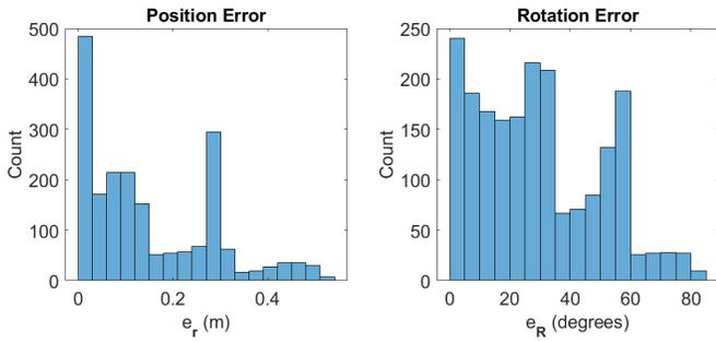
Fig. 3. Position and angle error in FDP (no end effector pose feedback provided)
