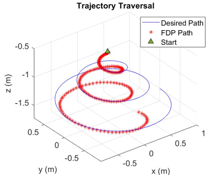
Fig. 2. Path of the manipulator solved using the FDP (no end effector pose feedback provided)
