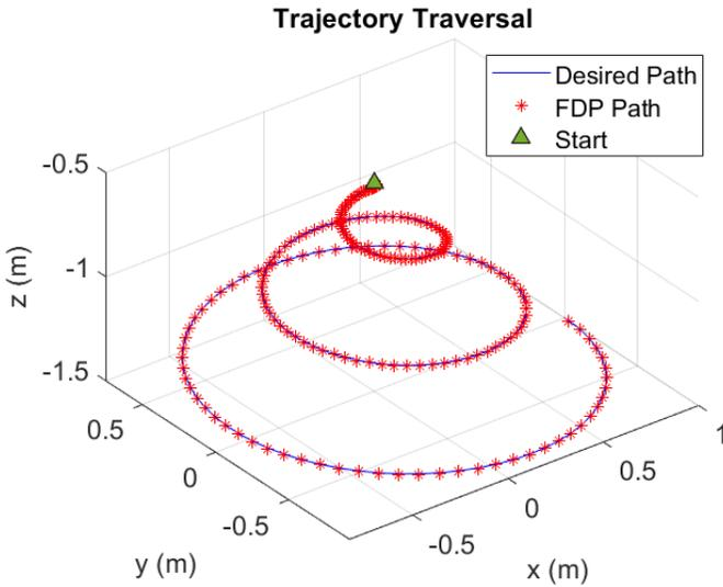
Fig. 4. Path of the manipulator solved using the FDP (end effector pose feedback provided)
