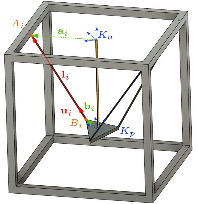
Fig. 1. Geometry of the hybrid CDPM with a central actuator and three surrounding cables
