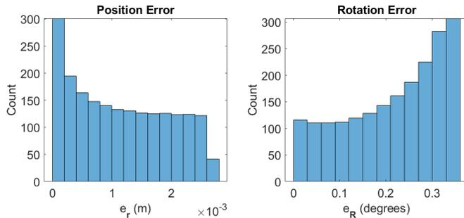
Fig. 5. Position and angle error in FDP (pose feedback provided to point algorithm toward the correct pose)
