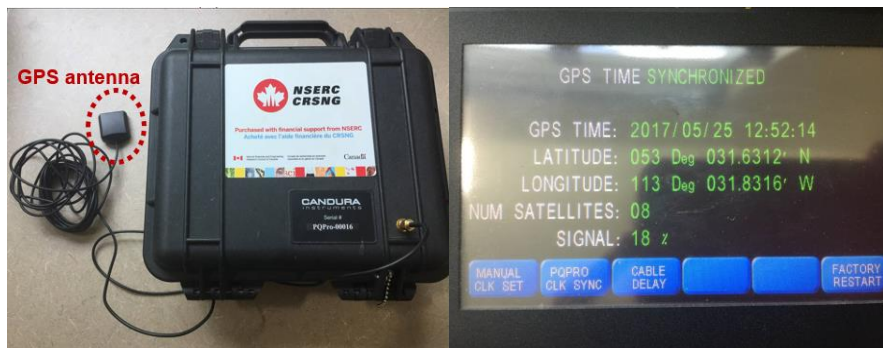
Figure 5.1 Portable power quality analyzer “PQPro”
