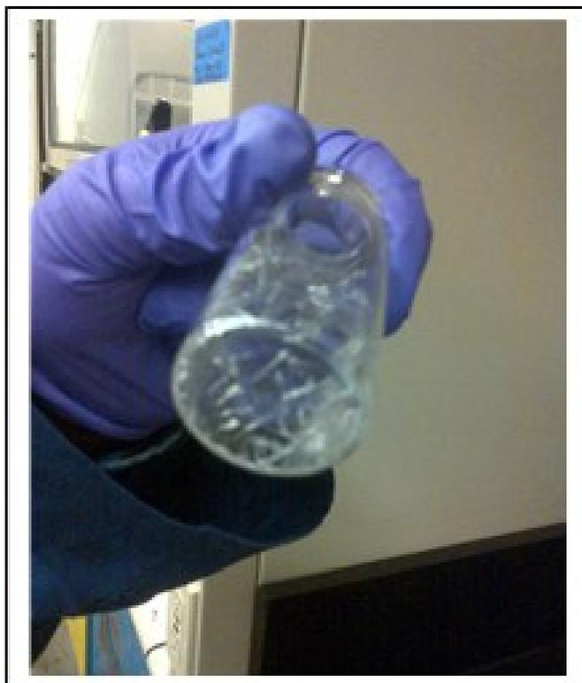
**Figure 4-11: Rod-like crystals of extracted Acenaphthene**
