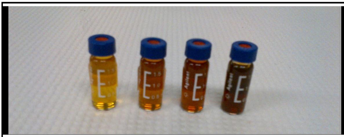
**Figure 5-2: From left to right: Coal Liquids derived at temperatures of 350, 400, 415, 450 °C and at residence time of 0 minutes**
