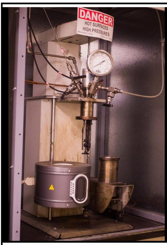
**Figure 3-1: High Pressure, High Temperature Stirred Reactor**
