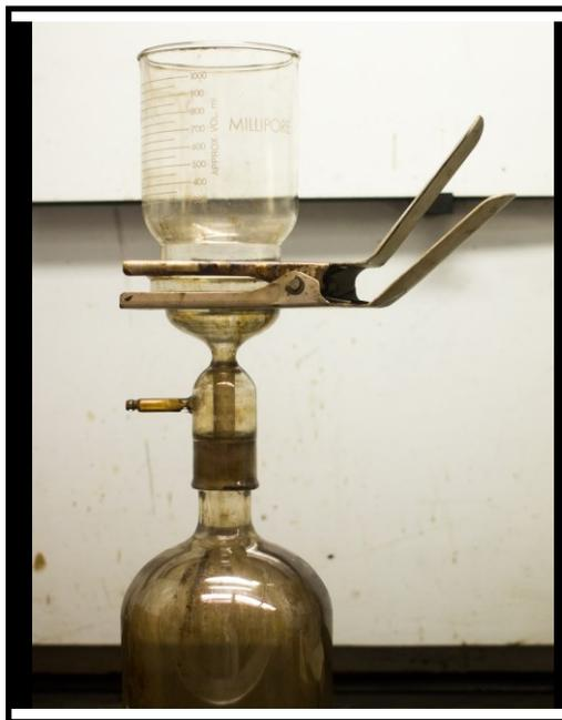
**Figure 3-2: Coal Liquid Filtering Flask Set-up**
