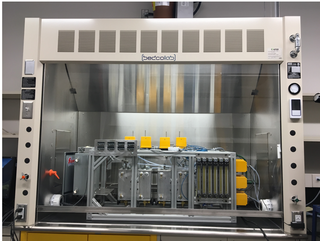
Figure 3.13: Sensor test rig setup in fume hood
