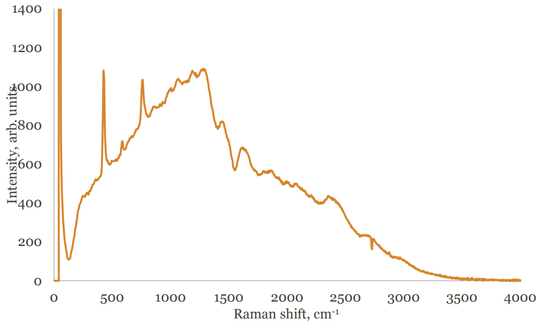
Figure 4-1: Raman spectrum of the sapphire window. The baseline of the signal can change throughout time.
