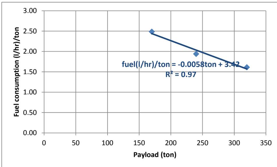
Figure 5-6: Relationship between DDC engines fuel consumption per ton and payload
