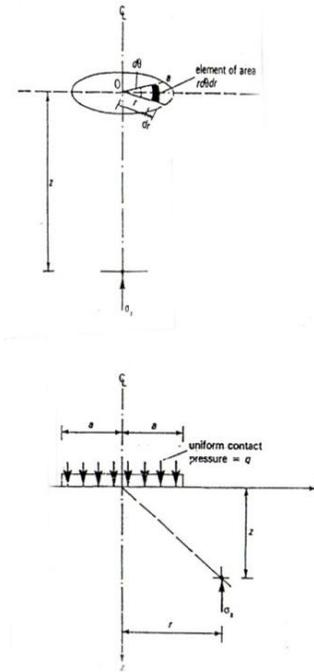
A 1 was used along with Boussinesq ground stress bulb to estimate stress variations with depth under the tire.
