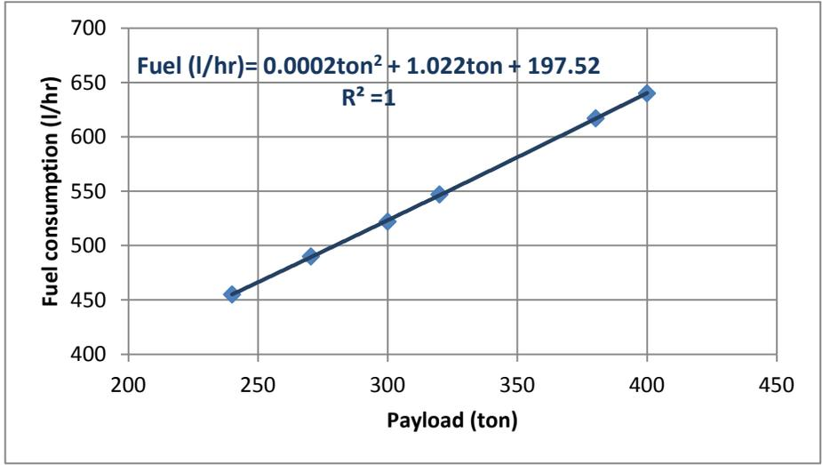
Figure 5-9: Relationship between Liebherr engines hourly Fuel consumption and payload
