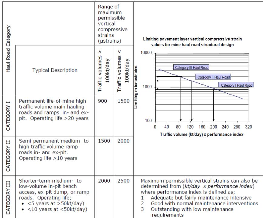
Figure 3-4: Typical haul road design categories and design data (after Thompson, 2011c )
