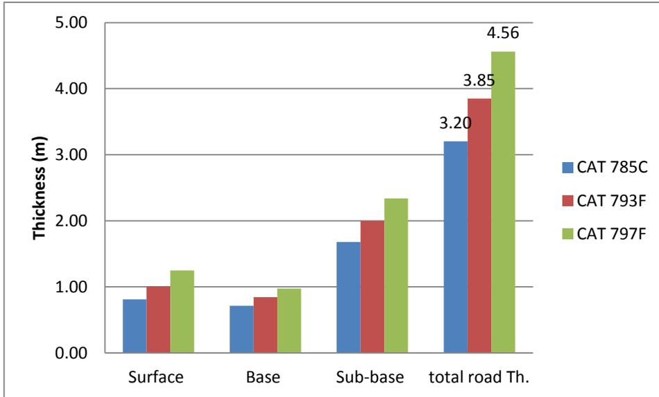
Figure 5-3: Road layers thicknesses for trucks
