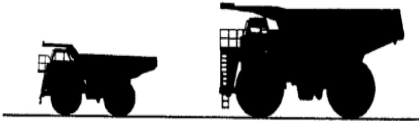
Figure 2-2: Comparative profiles of 400ton and 100ton capacity trucks (Caterpillar, 1999)
