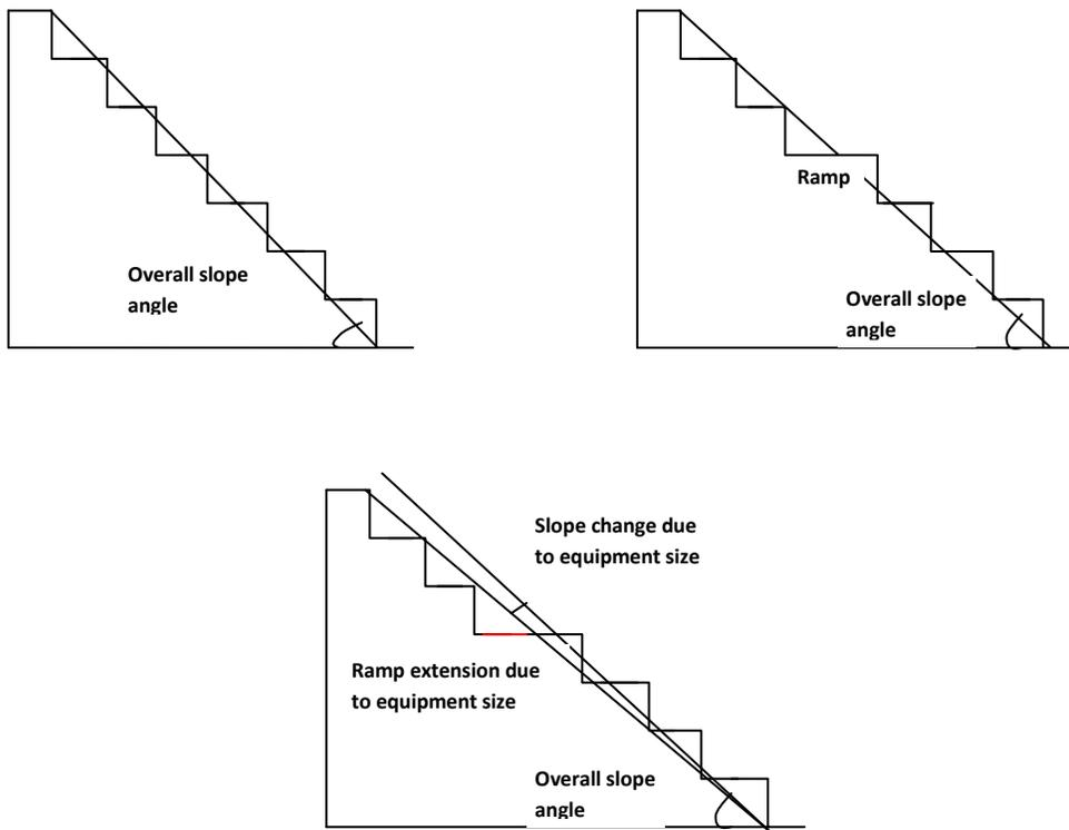
Figure 3-1: Effect of equipment size on pit slope (After Bozorgebrahimi 2004)
