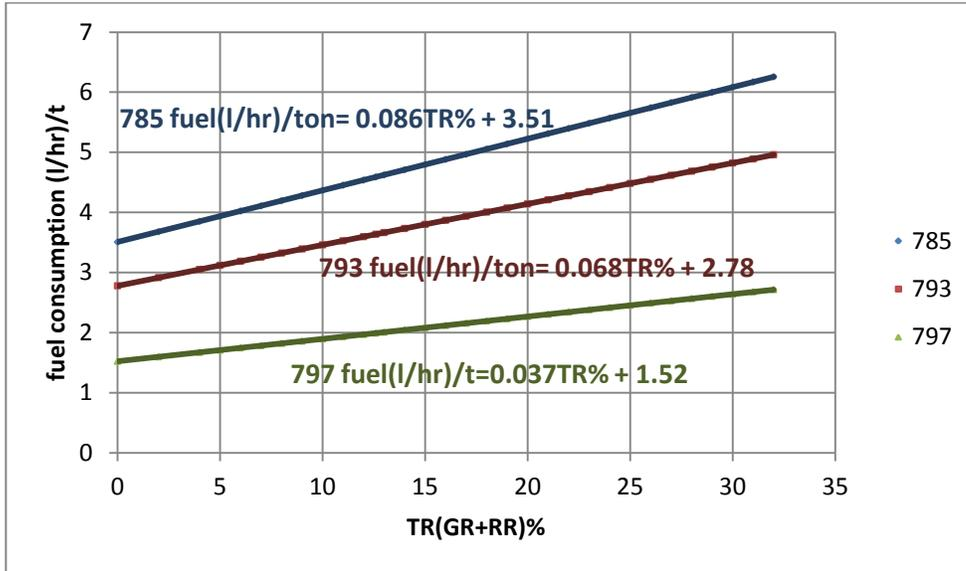
Figure 5-15: Relationship between TR and fuel consumption per ton
