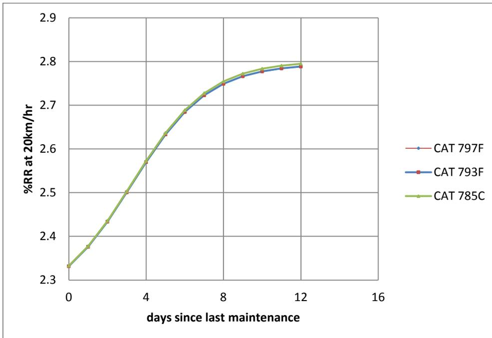
Figure 5-5: Trucks rolling resistance progression in 12 days
