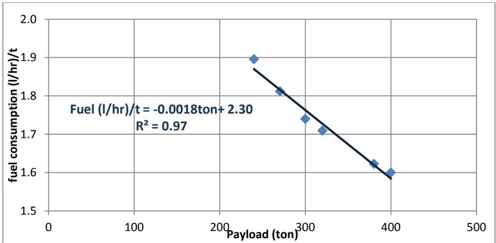
Figure 5-8: Relationship between Liebherr engines fuel consumption per ton and payload
