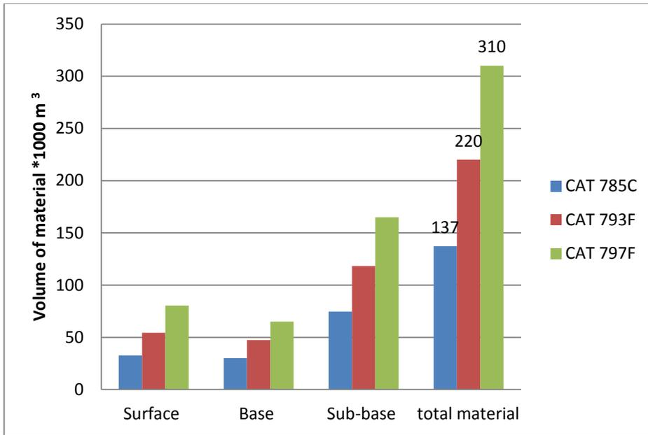
Figure 5-4: Construction materials requirement
