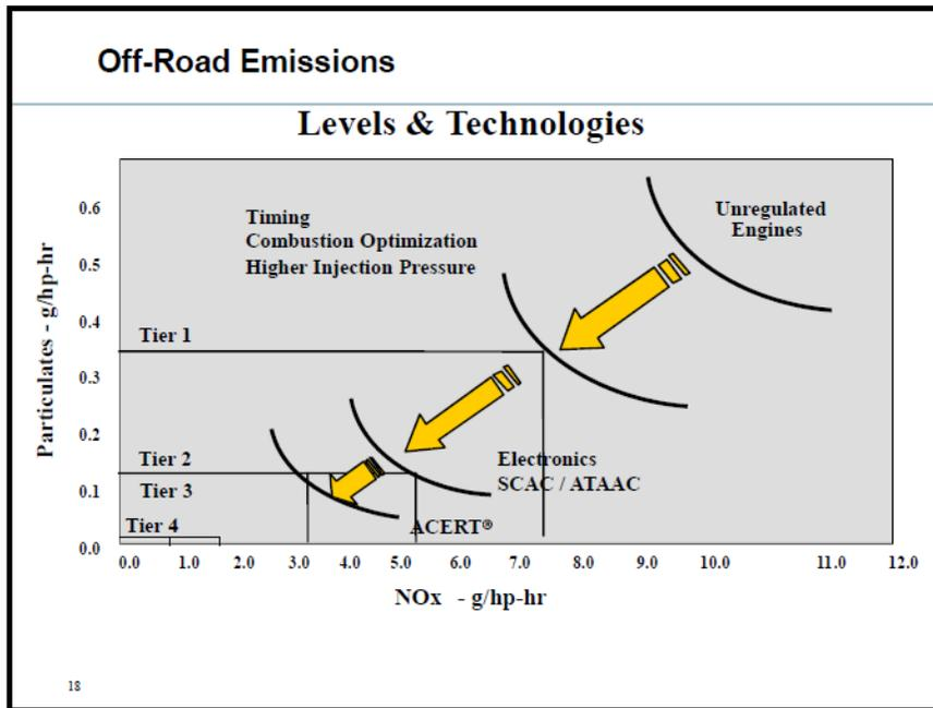
Figure 5-10: Emission control in tier engines (Caterpillar, 2008).
