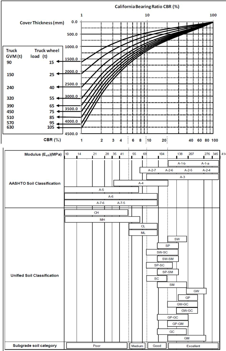
Figure 3-3: CBR cover curves for 90-630 metric ton GVM haul trucks and approximate bearing capacities of various soil types defined by UCS and AASHTO systems(after Thompson 2010)
