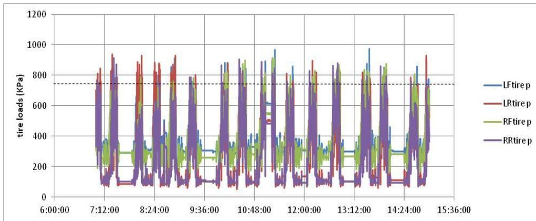
Figure 5-1: Tire loads in field operation
