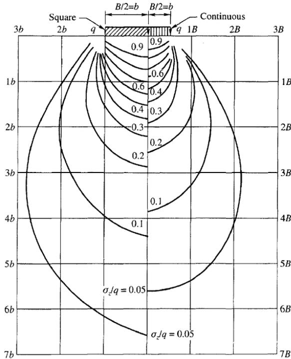
Figure 3-5: Boussinesq ground stress bulb ( after Perloff, 1975).
