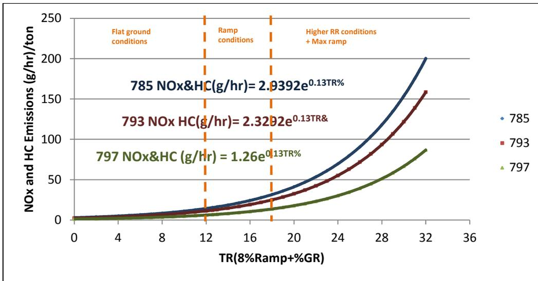
Figure 5-16: Relationship between TR with HC and NOx emissions for different truck sizes
