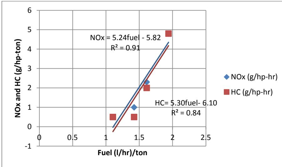
Figure 5-11: Relationship between fuel consumption with NOx and HC emissions.
