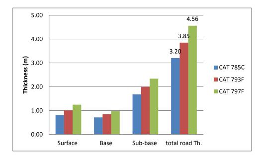
Figure 5-3: Road layers thicknesses for trucks
