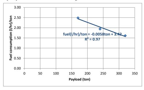
Figure 5-6: Relationship between DDC engines fuel consumption per ton and payload
