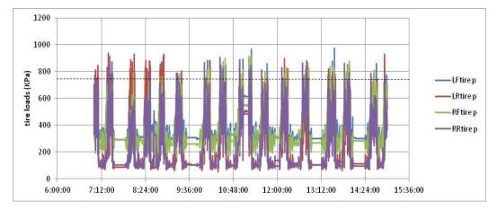
Figure 5-1: Tire loads in field operation
