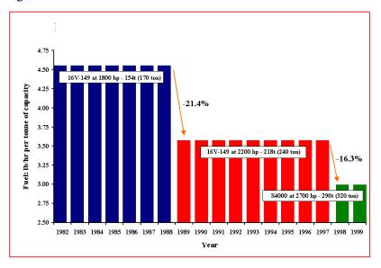
Figure 4-1: DDC Fuel consumption per ton of truck capacity (After Leslie, 2000)
