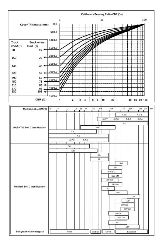
Figure 3-3: CBR cover curves for 90-630 metric ton GVM haul trucks and approximate bearing capacities of various soil types defined by UCS and AASHTO systems(after Thompson 2010)
