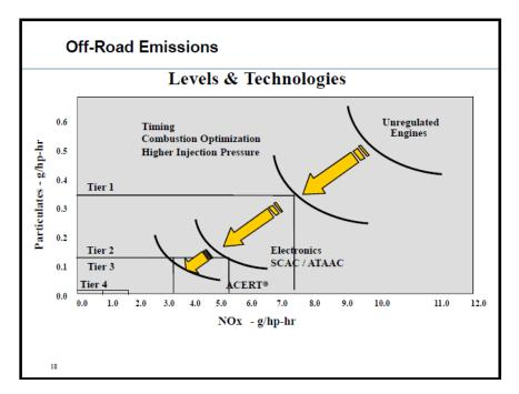
Figure 5-10: Emission control in tier engines (Caterpillar, 2008).
