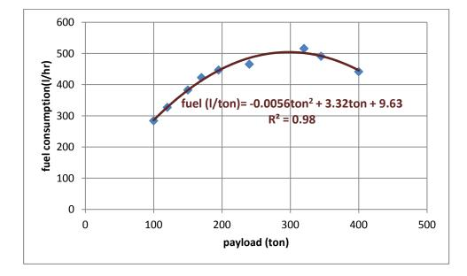
Figure 5-7: Relationship between DDC fuel consumption and payload
