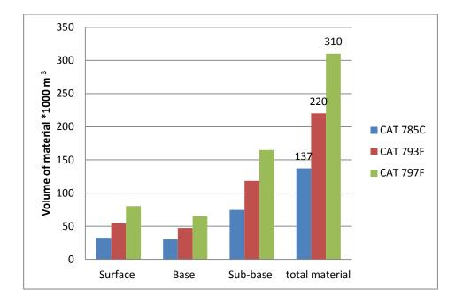
Figure 5-4: Construction materials requirement
