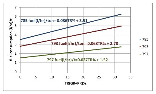
Figure 5-15: Relationship between TR and fuel consumption per ton
