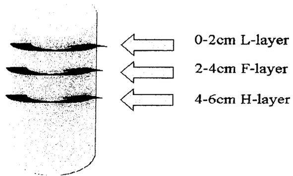
Fig. 4.5. Diagram of a soil core showing the stratification into 2 cm layers for further analysis.
