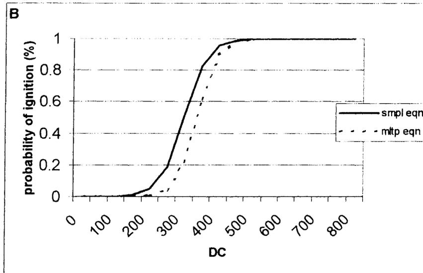
Figure 4.6. Results of the non-linear analysis fitted to a logistic model showing the probability of sustained ignition against the DMC (A) and DC (B). Model predictions at the 50% probability for either the simple/multiple equations for DMC are 27/29, and for DC are 300/336. For DMC (A), and2000 (Anderson 2000) shown for comparison.
