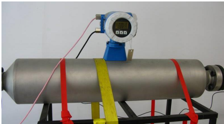
Figure 19 - Coriolis meter with bundled 4-20mA outputs (pink)
