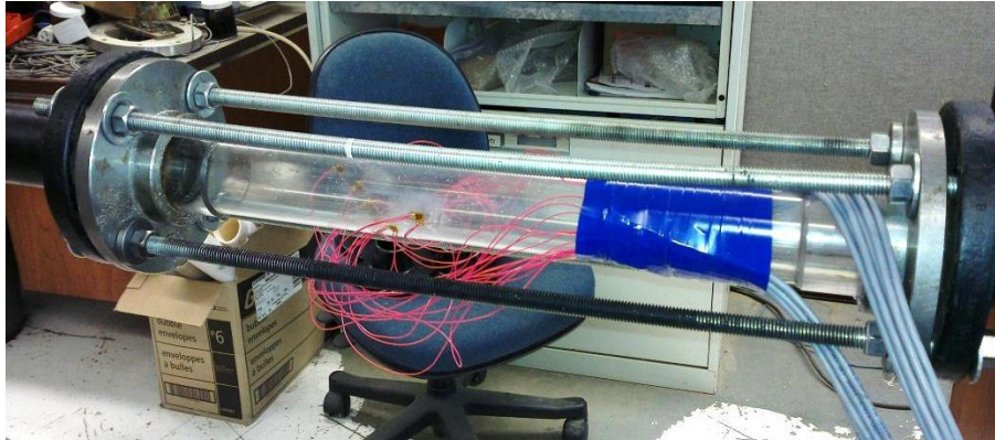
Figure 22 - Strain spool with eight rosettes spaced 25.7° apart
