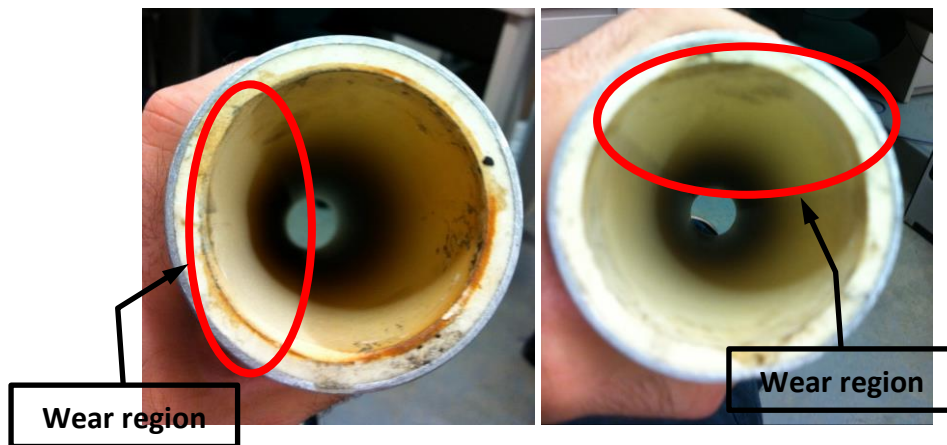
Figure 41 - Sample wear specimens after undergoing testing
