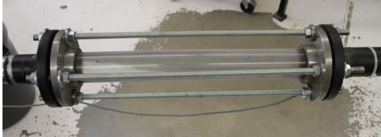
Figure 17 - Removable test section with clear viewing tube and axial preload support rods
