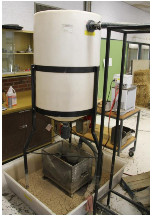
Figure 16 - Waste tank, sieve box, and catch bin
