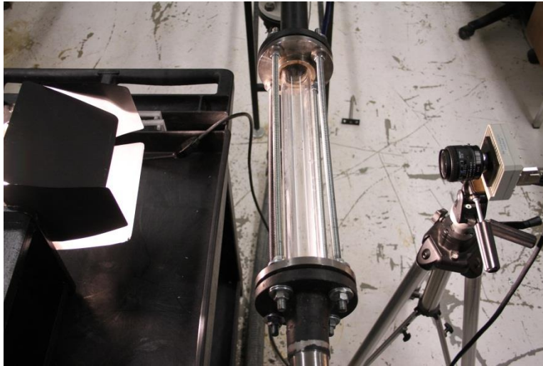
Figure 26 - Setup for optical particle-tracking experiments
