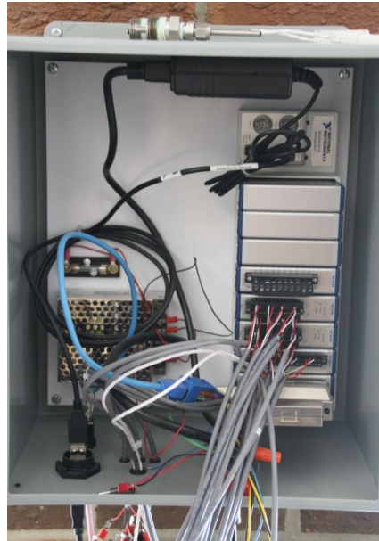
Figure 18 - DAQ with external power supply
