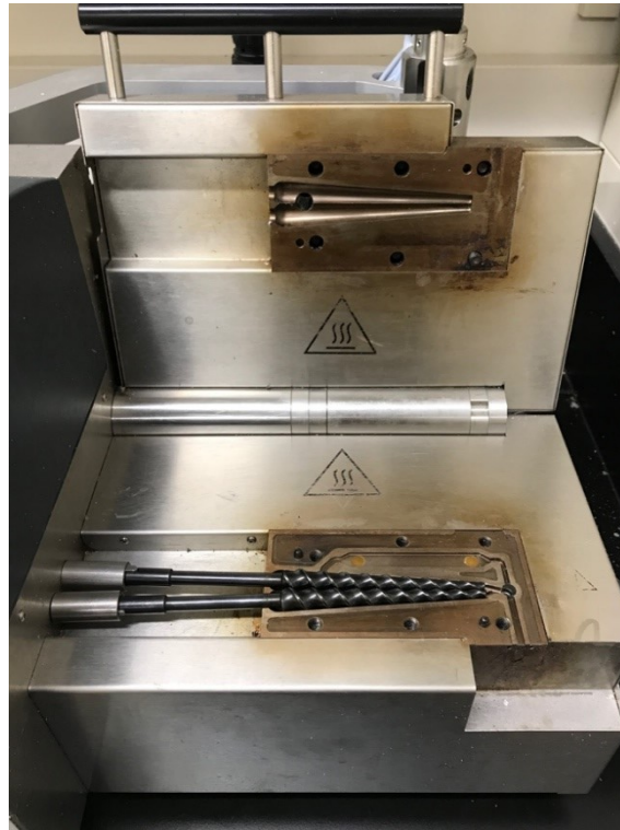
Figure 3.1: HAAKE Minilab II micro compounder with a conical twin-screw setup
