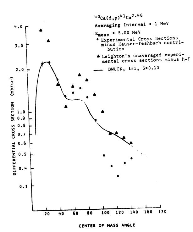
Yield curve of 40Ca(d,p) leaving 41Ca in ground state, first and third excited states. Cross sections are averaged over 50 keV. Measurements were made at an angle near the stripping peak.
