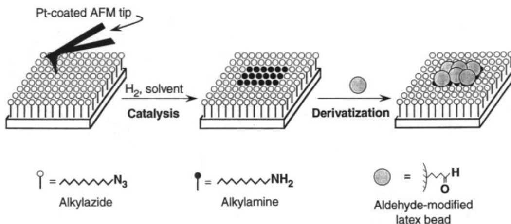
Figure 1.12. Schematic of site-selective hydrogenation of an azide-terminated surface using a Pt-coated AFM tip in the presence of hydrogen. The newly formed amino groups were then used to assemble aldehyde-modified latex beads. Reprinted with permission from ref. 62.
