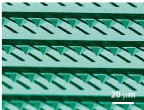
Figure 1.6. An SEM image of a portion of a 2D array of 55,000 AFM tips. Reprinted with permission from ref. 48b. Copyright © 2007 American Chemical Society.
