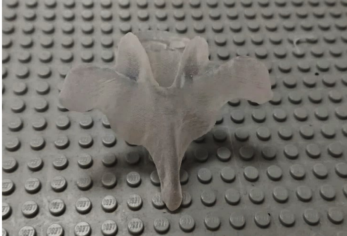
Figure 6-7: 3D-printed T6 phantom for ultrasound scans
