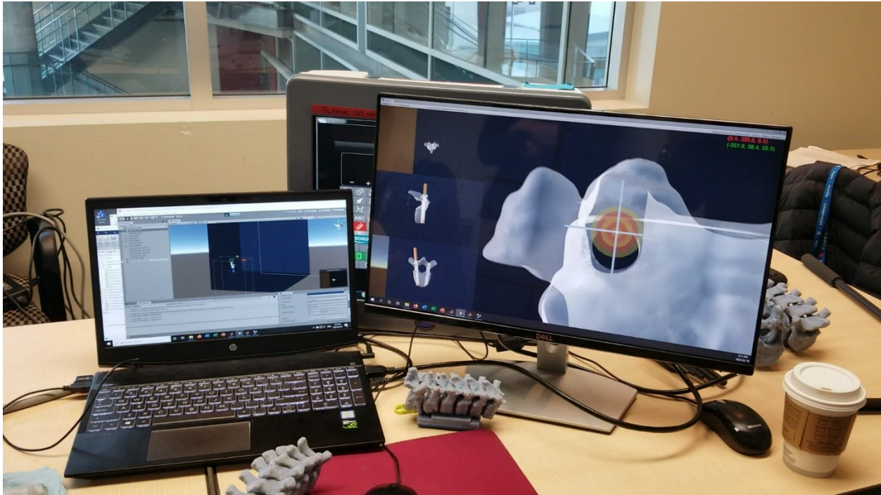
Figure 7-31: Navigation display showing pedicle probe (yellow/red cylinders) placed into pedicle holes
