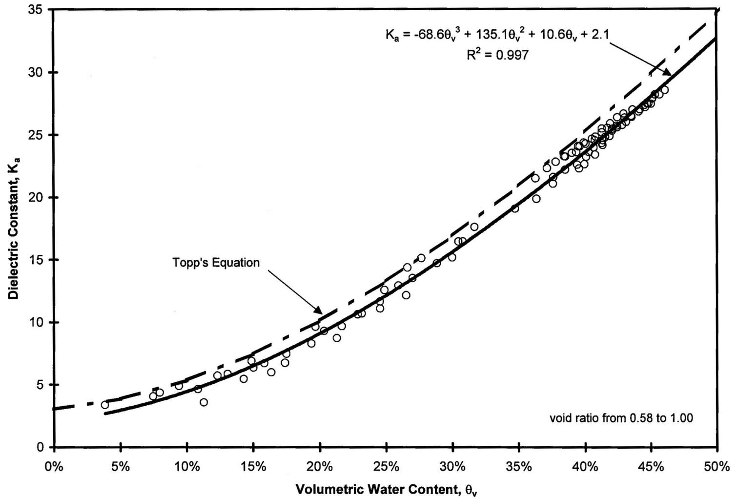
Figure 4 - Apparent dielectric constant versus volumetric water content.
