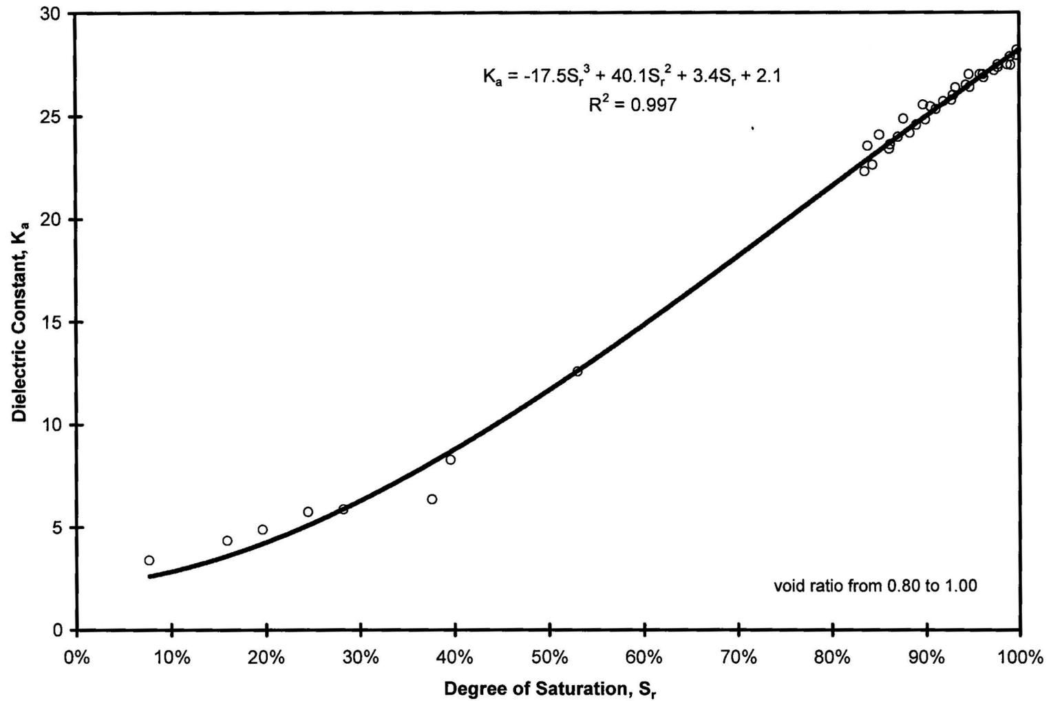
Figure 6 - Apparent dielectric constant versus degree of saturation for void ratios from 0.80 to 1.00.
