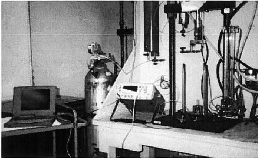
**(a) TDR setup triaxial tests**
