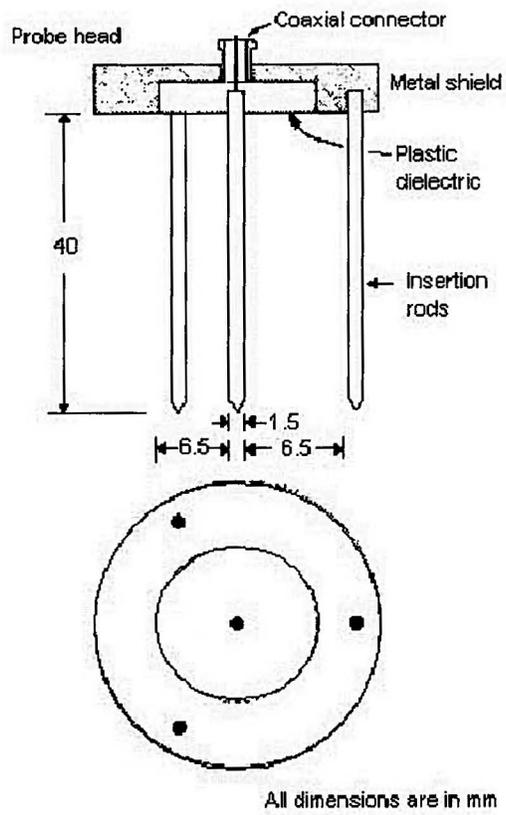
**Figure 2 - TDR probe geometry.**
