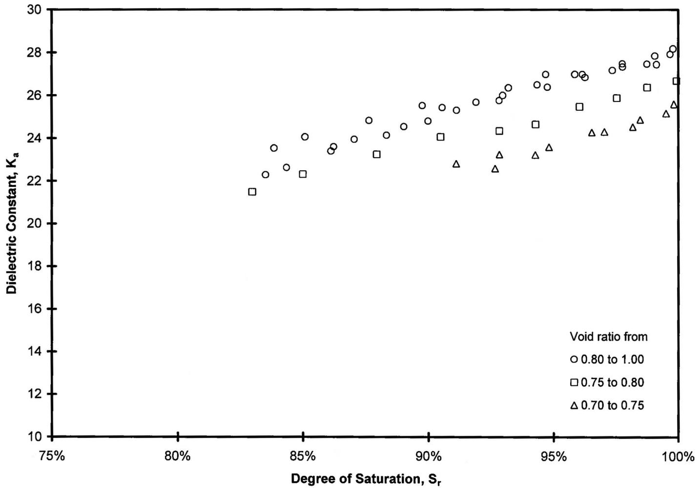
Figure 5 – Apparent dielectric constant versus degree of saturation.
