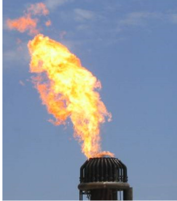
Figure 1.4: External air ring flare tip design reproduced from Smith and Seefeldt [24] with permission from Zeeco, Inc.
