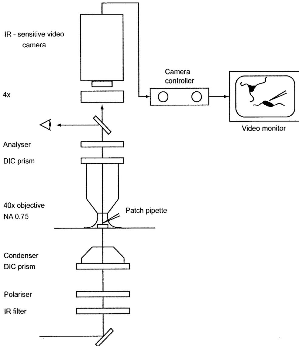
**Figure 2-5.** Diagram of the Zeiss Axioskop FS used for visualizing substantia gelatinosa neurons. The microscope is mounted on two linear actuators, allowing the microscope to be moved in the  $x$ - and  $y$ -axes, without affecting the relative position of the recording and stimulating electrodes. The recording chamber is mounted on a separate fixed stage.
