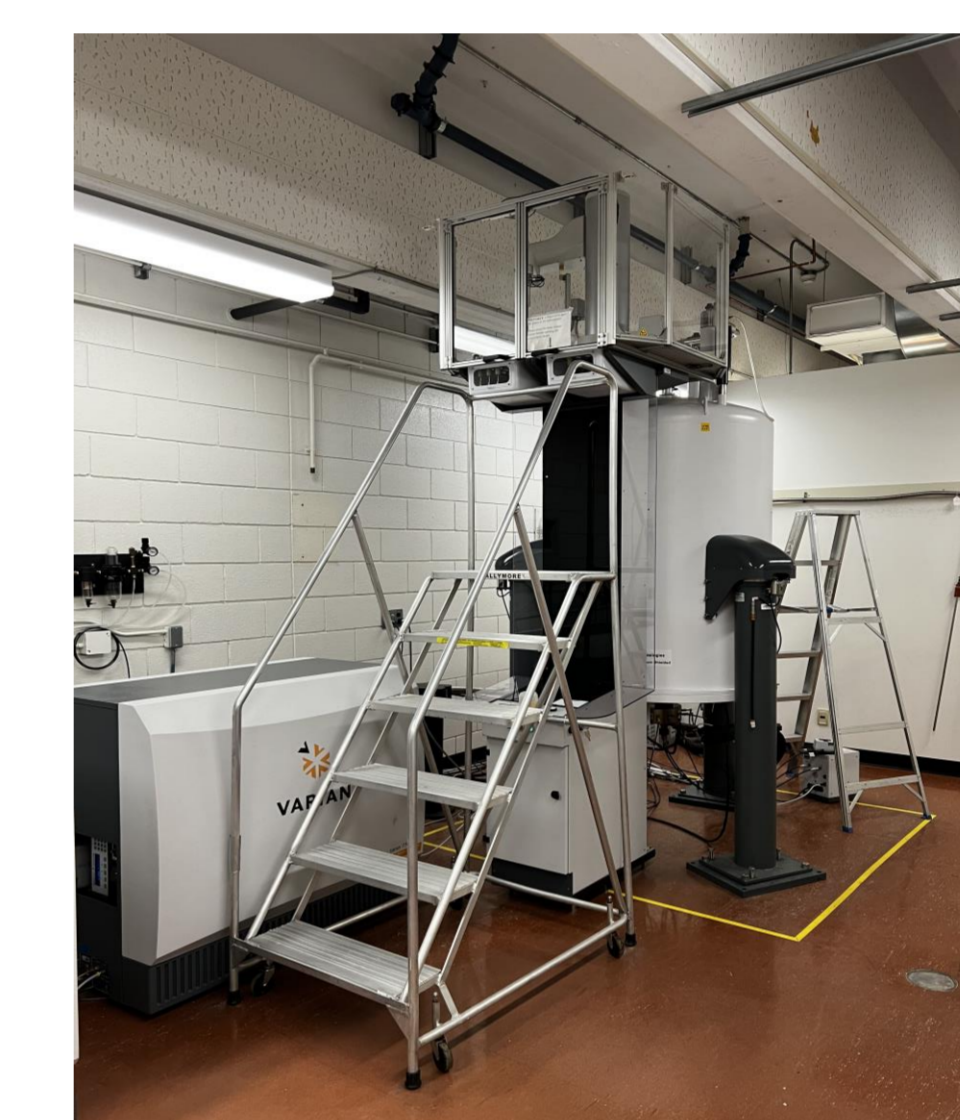
Figure 4. An instrument used for NMR (Nuclear Magnetic Resonance) spectroscopy to identify molecules and assess their purity. Results presented on the right were obtained from the NMR instrument.
