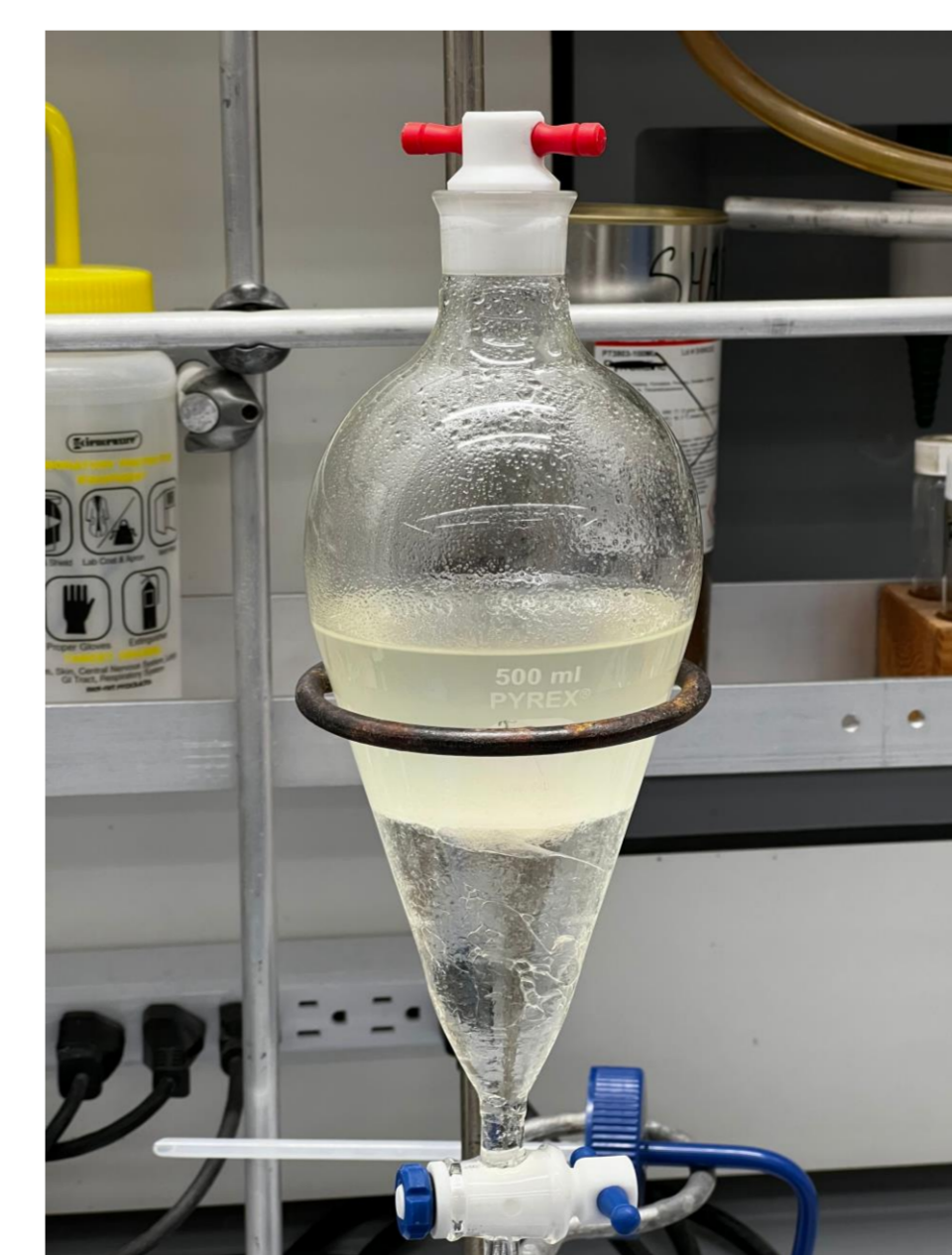
Figure 3. Aqueous Workup being done for removal of aqueous soluble substances, for instance water, present in an organic solution.
