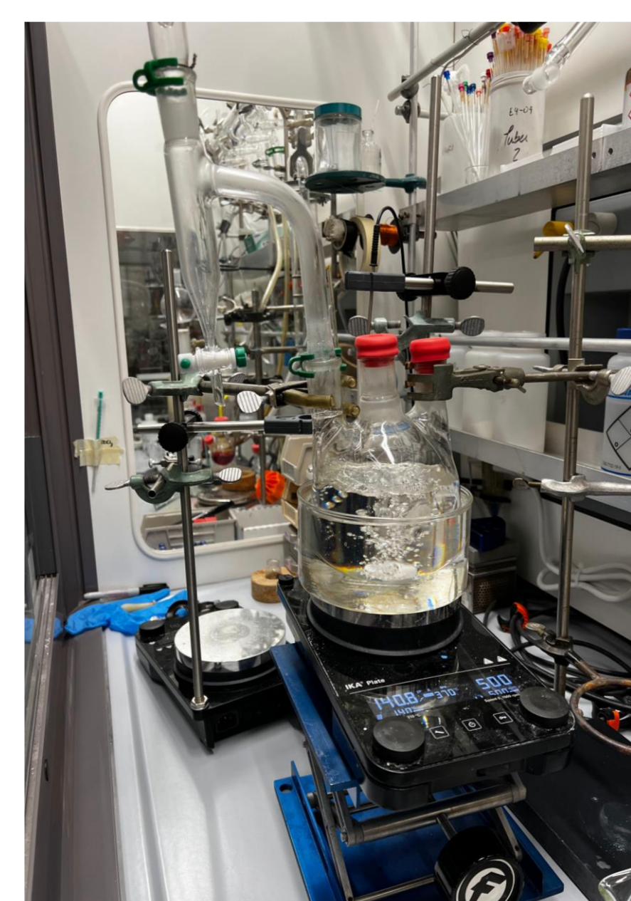
Figure 2. Reaction setup employing the use of a Dean-Stark trap, a piece of glassware designed for removal of water.
