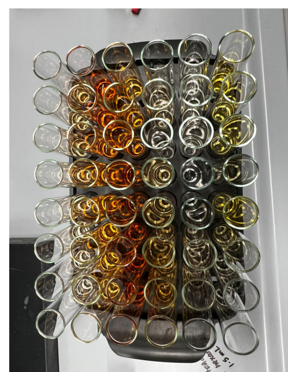
Figure 1. Samples obtained from silica column chromatography using the Biotage automated flash chromatography instrument.
