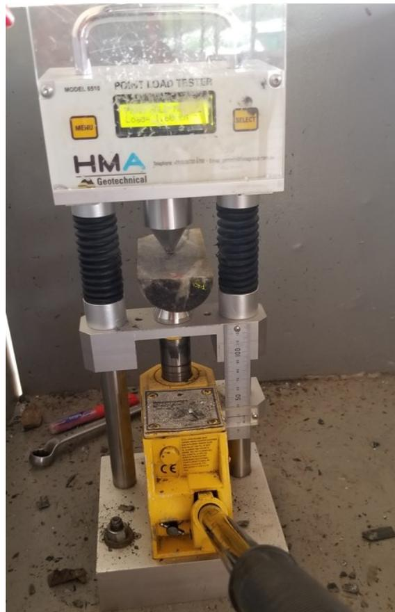
Figure 4-7: Point Load Strength index test setup
