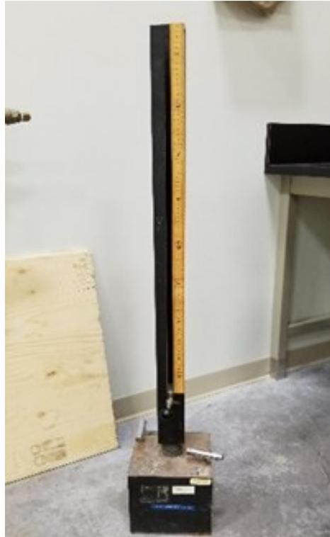
Figure B8-5: Drop weight test setup
