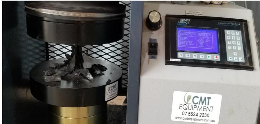
Figure 4-3: Uniaxial compressive strength test setup
