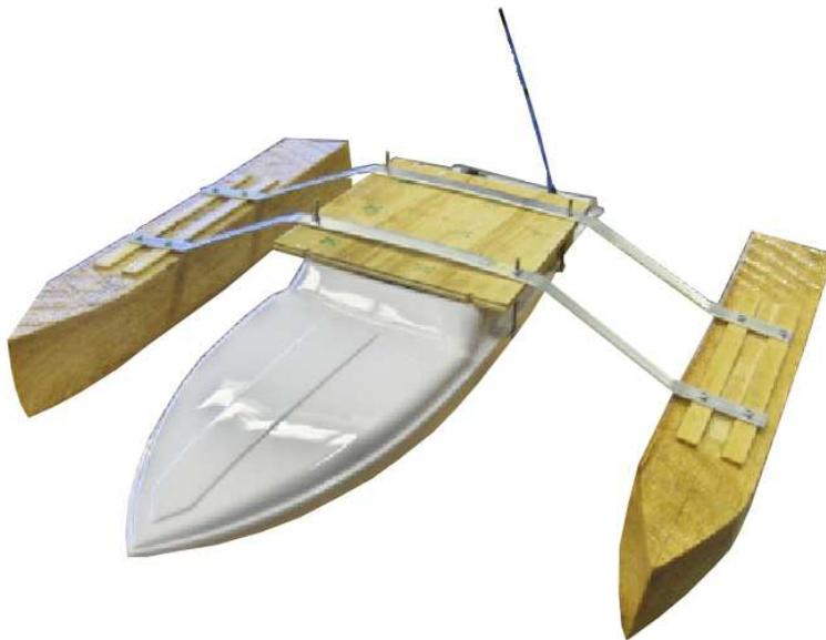
Figure 4.7: The Complete Assembly on the Boat
