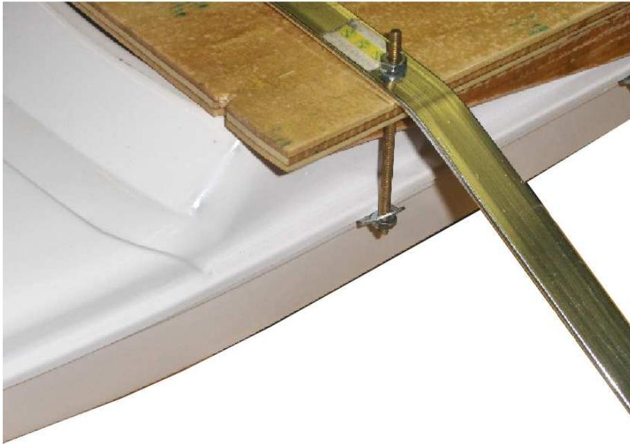
Figure 4.6: Close view of Clamps used to Fasten Boat Mount to the Hull of the Boat
