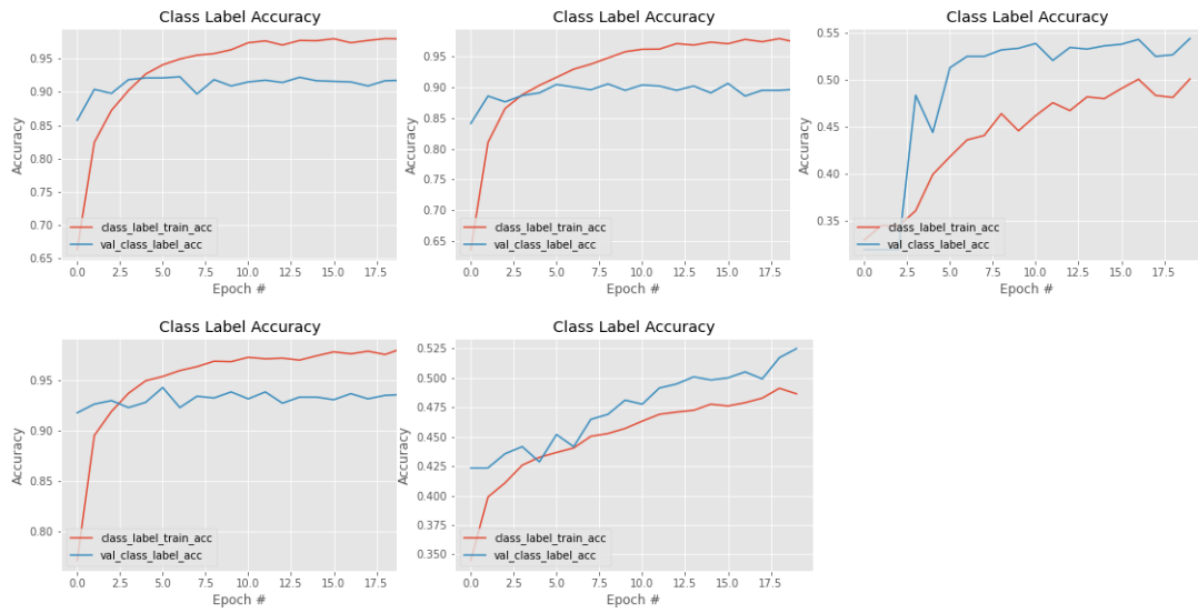
Figure 5.5: Training-Validation accuracy over the epochs for VGG16, VGG19, ResNet50, DenseNet201, and MobileNetV3Large
