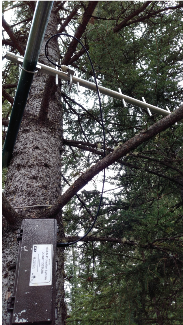
Figure D.16: Photograph of a signal repeater connected by a cable to a high-gain Yagi-Uda antenna. These antennas were used at some sites to increase the reliability of connections between tree-mounted devices.
