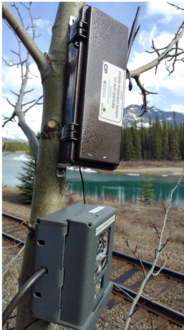
Figure D.5: Photograph of a tree-mounted box enclosure (camera controller, upper) along with a Reconyx camera (lower). The black line between the two is the external trigger cable for the camera.
