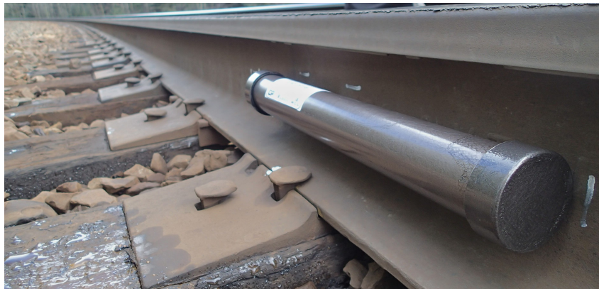
Figure D.1: Photograph of the tube enclosure (a train detector) attached to the railway track.
