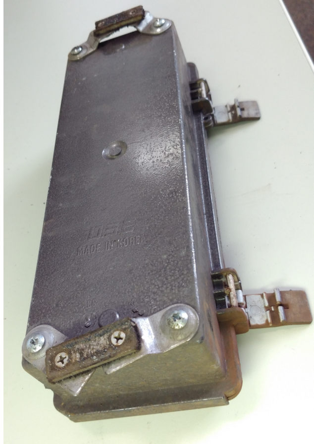
Figure D.4: Photograph of the track-facing side of a box enclosure (a train detector). This image was taken following field service, so the magnets and other surfaces are covered with iron filings and dust.
