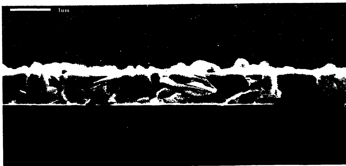
Figure 3.15: Microstructure of thin film \text{Bi}_2\text{Te}_3 deposited at a Te:Bi flux ratio of 2.3:1.
