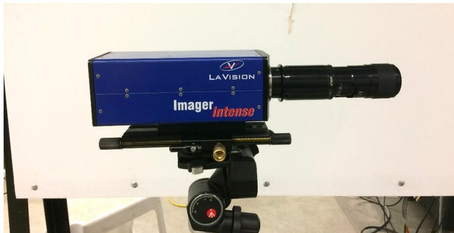
**Figure 3-9. LAvision image intense double framed camera with 12x Navitar lens**
