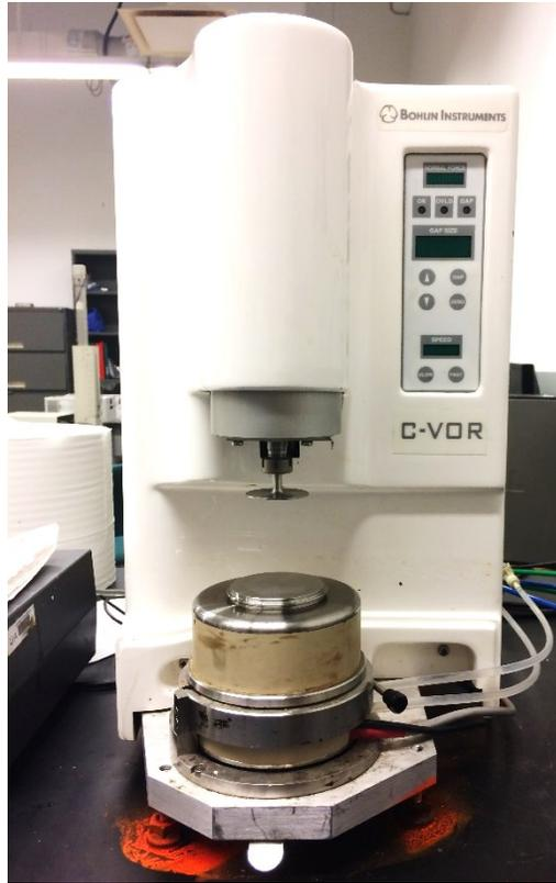
**Figure 3-4. Bohlin rheometer**
