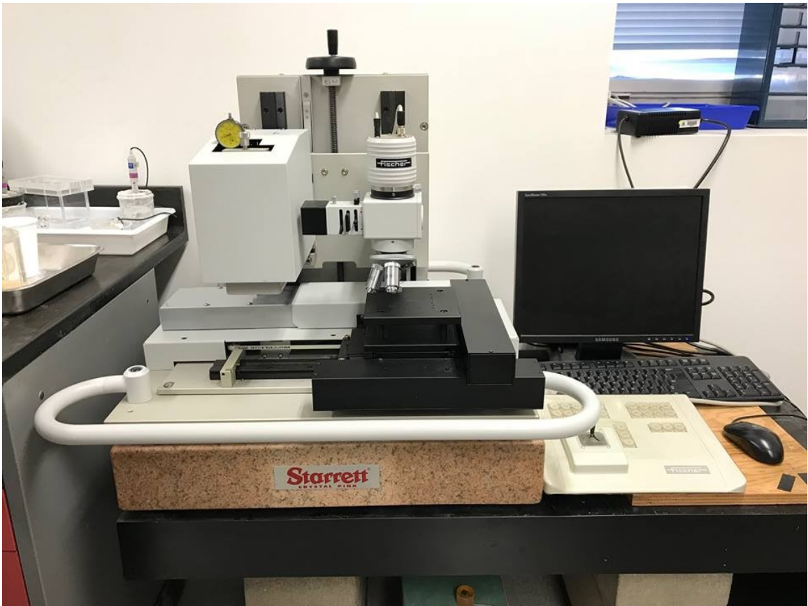
Figure 3.5 Vickers micro-hardness tester (Fisherscope H100C Microhardness Measurement System with WIN-HCU software)
