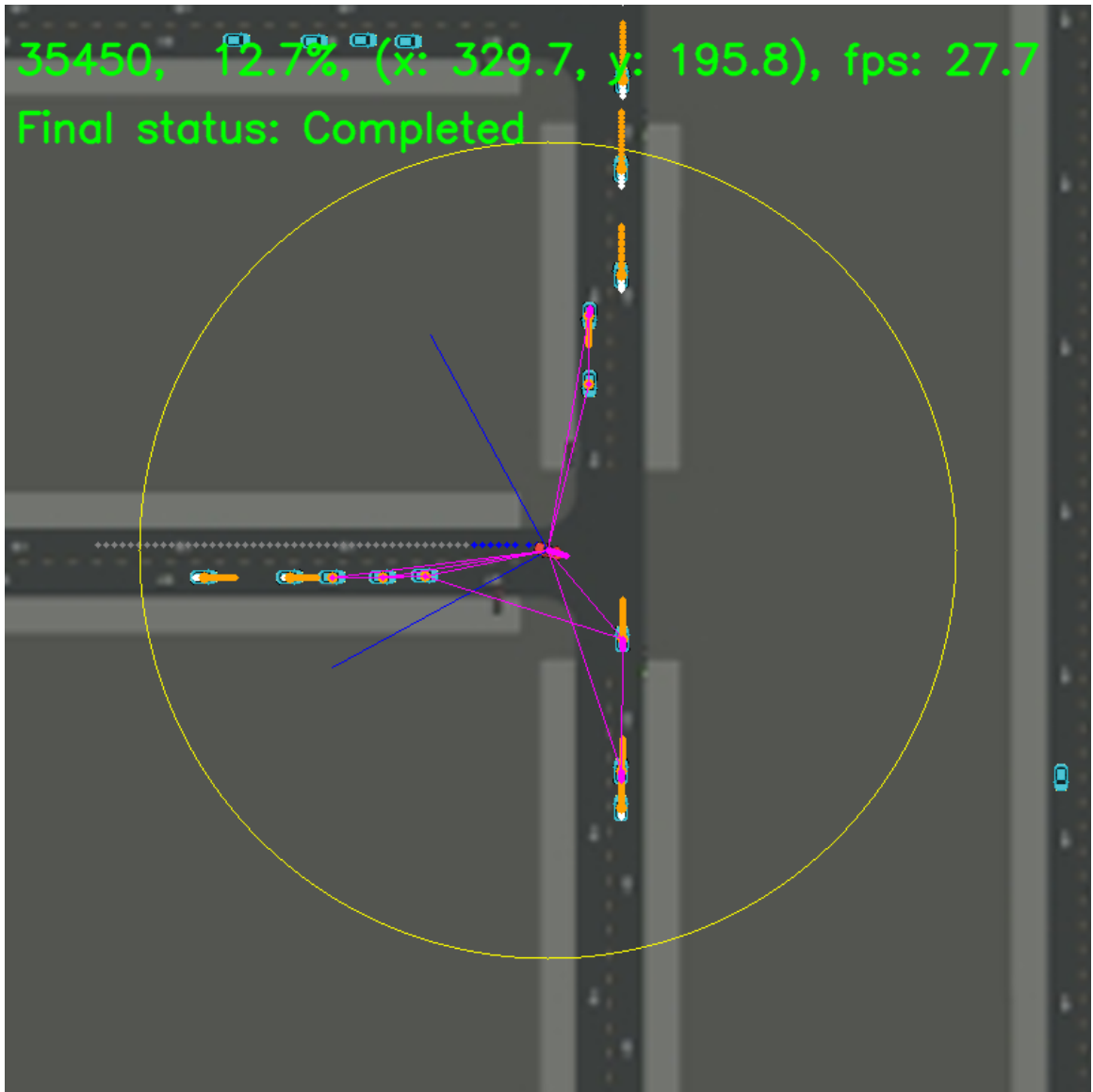
Figure 2.4: A screenshot of the Visualizer. We developed the visualizer for inspecting the recorded driving data during the Carla Autonomous Driving Challenge. The figure shows a bird's-eye view of the traffic situation centered at the top of the ego vehicle, the two blue line segments for the FOV, and the yellow circle indicates the communication range between the ego vehicle and the surrounding CAVs. Orange dots and lines represent the detected position and predicted future trajectories of the nearby obstacles. Blue dots denote the local waypoints, and gray dots denote the global waypoints. Finally, the connectivity between CAVs is shown in purple.
