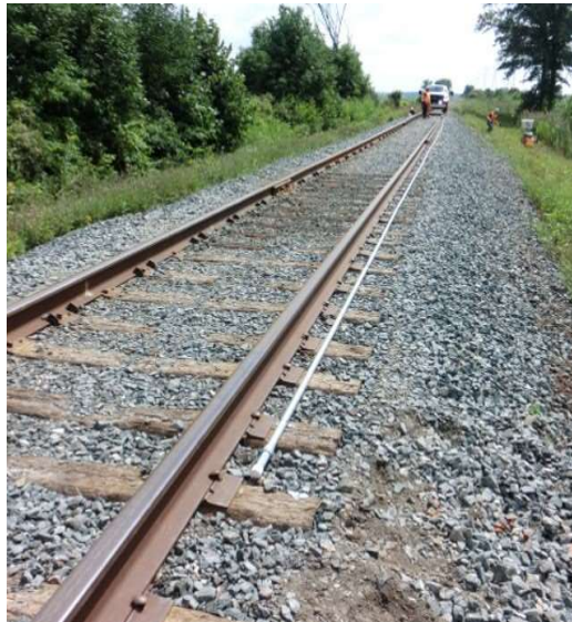
Figure 2.7: ShapeArray SAAX Railroad Application (Courtesy of Measurand Inc.)
