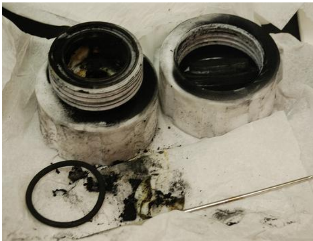
Figure 3.18. Damaged Teflon container. Photograph by Jeffrey N. Murphy, licensed under the Creative Commons Attribution 3.0 Unported (CC BY 3.0) license. 28
