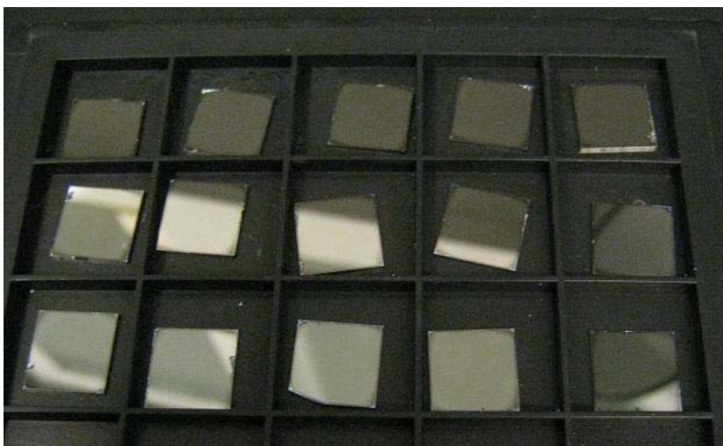
Figure 2.4. Picture of block copolymer thin film-coated silicon substrates. The silicon substrates are 1 cm by 1 cm in size.
