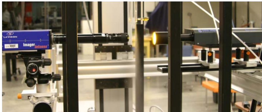
Figure 3-3. An image of the Shadow-PTV system.
