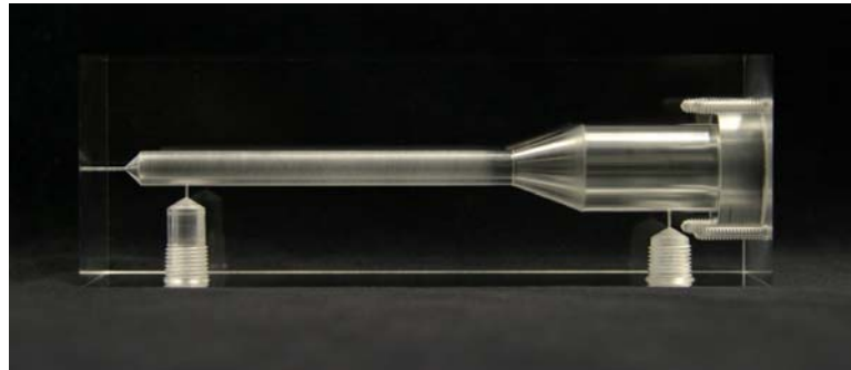
Figure 2-6. An image of the effervescent atomizer mark I made from cast acrylic.
