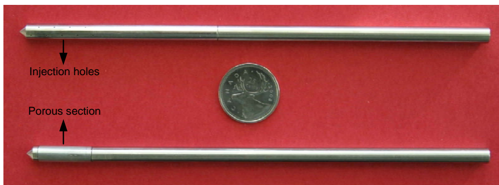
Figure 2-9. An image of the two air injectors used in the second effervescent atomizer.
