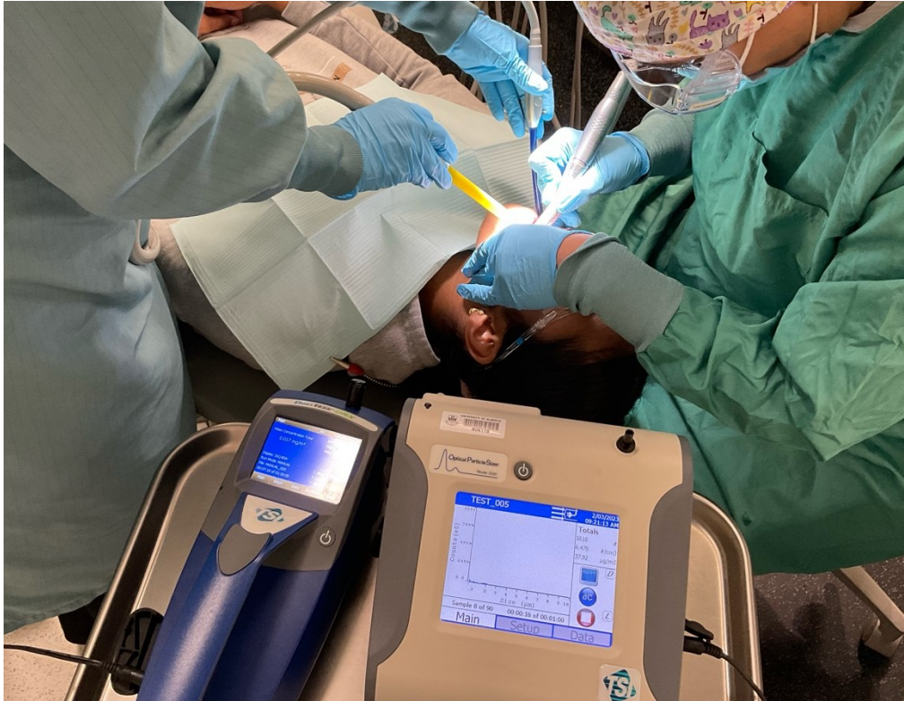
Figure 11 - OPS and Dust-Trak positioning in a Sampling Session.
