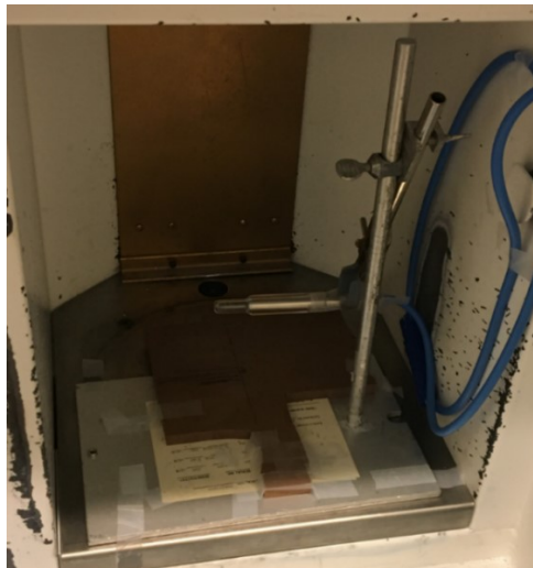
Figure 5.4: Configuration of the ion chamber, with the 2 mm acrylic buildup cap, during calibration in the Cs-137 irradiator. The PTW 30013 ion chamber is held by a retort stand and clamp, which is fastened to the turntable with single-sided and double-sided tape (underneath the stand’s base).
