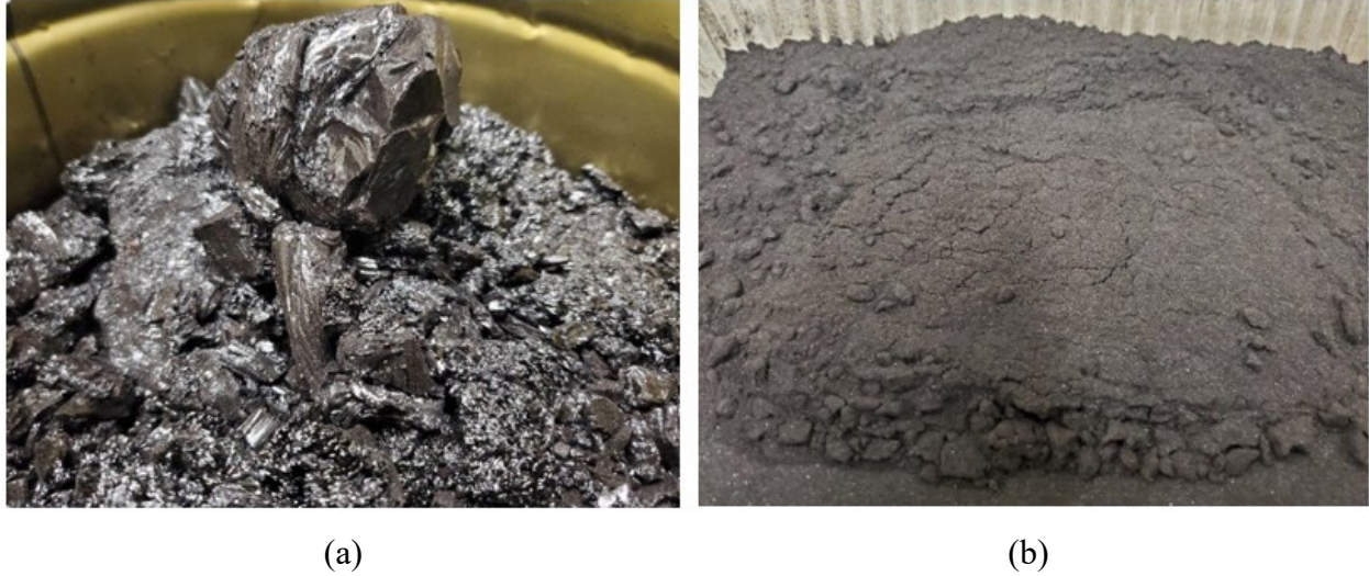
Figure 2-17. Asphaltenes: (a) Solid Form; (b) Powder Form after Passing through a #100 Sieve
