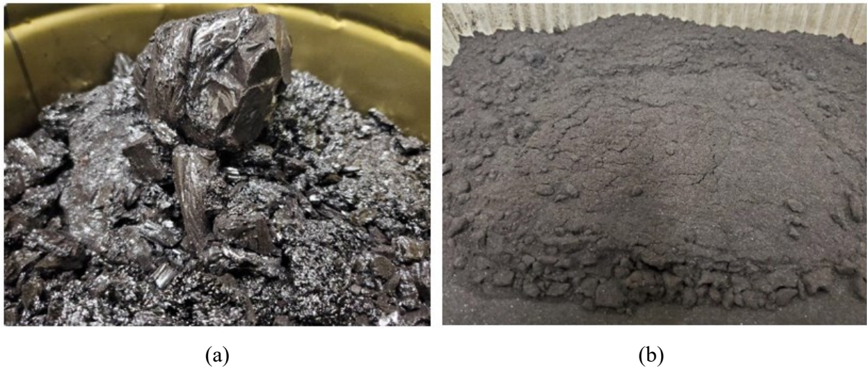
Figure 3-1. Asphaltenes: (a) Solid form; (b) Powder Form After Passing Through a #100 Sieve
