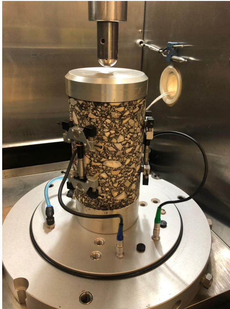
Figure 2-5. Dynamic Modulus Test Setup in UTM
