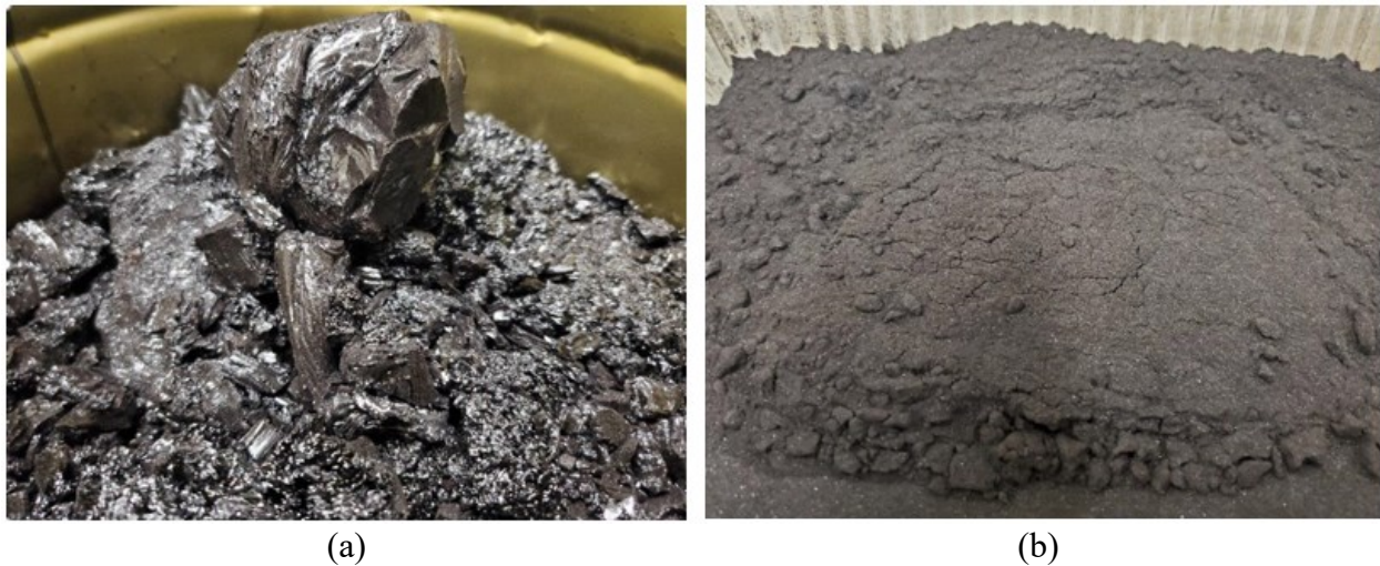
Figure 4-1. Asphaltenes: (a) Solid Form; (b) Powder Form after Passing through a #100 Sieve
