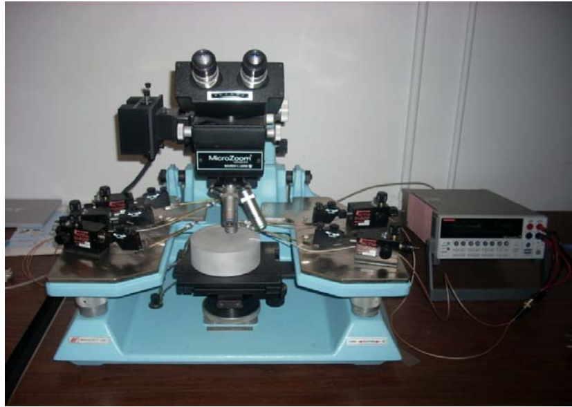
Figure 3.7: Device Test Rig with Keithley 2400 Source
