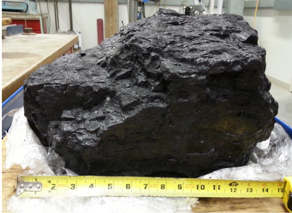
Figure 4.2 A coal block from the Genesee coal mine in the Central Alberta, Canada *Note: The measuring tape's divisions are in inches.
