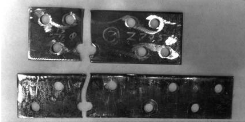
Figure 4.10 – Fatigue crack patterns for specimens Gb (top) and S2a2 (bottom).
