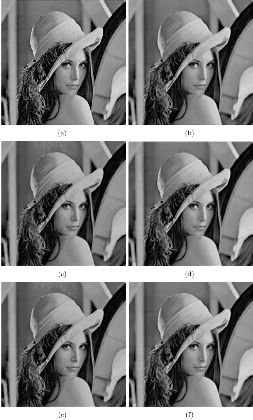
Figure 4.15: Image smoothing (a) original image (b) using an accurate multiplier (c) using an 8/4 AM1 (d) using an 8/8 AM1 (e) using an 8/4 AM2 and (f) using an 8/8 AM2.
