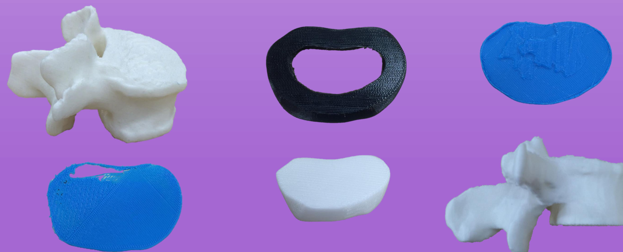
Figure 3 – The individual pieces of the lumbar model. In blue: the cartilage endplates. In black: the annulus fibrosus. In white: the two vertebrae and the nucleus pulposus. Individual parts not to scale.
