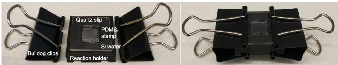
**Figure 2.15** Photograph of a customized experimental setup for plasmonic stamping: a silicon wafer was stamped with a plasmonic stamp and sandwiched between a quartz coverslip and a customized reaction holder, which was made of polytetrafluoroethylene (PTFE). Two clips were applied on both sides of the sandwich structure.
