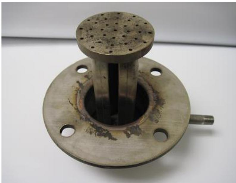
**Figure 4-3 Impact plate at the bottom of the drop tube furnace.**
