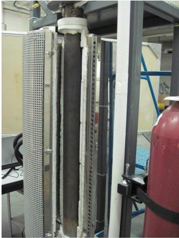
Figure 4-5 Tube reactor inside a partly opened split vertical tube furnace.
