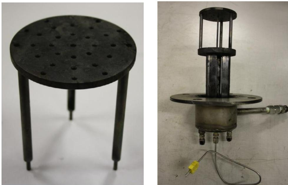
**Figure 4-4 New impact plate (left) and modified impact plate assembly (right).**
