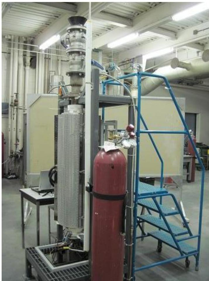
**Figure 4-2 Drop tube furnace for drop test at high temperature.**
