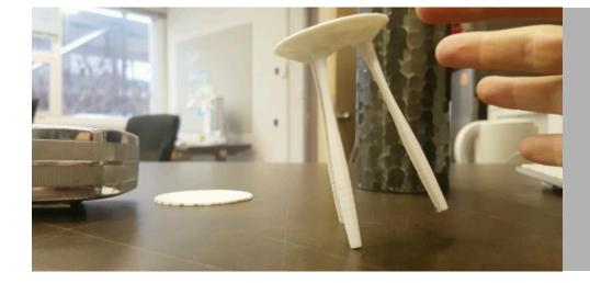
3D printed models of taller versions of the first stool demonstrated that increasing the leg lengths without changing the seat component made the taller stools less stable
