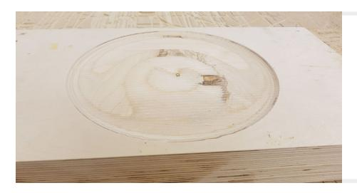
Adding a concave to the top of the seat added complexity to the milling operations. The wood stock now had to be milled on two faces. The concave surface of the seat was milled first.
