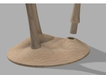
The initial stool featured a flat seat with a contoured surface underneath. The contoured surface of the seat component was designed to be milled from a solid block of wood. The milling process included three operations and two tool changes.
