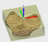
Milling this component from a solid block of wood wastes more that 50% of the material. On a 3-axis CNC, milling this component from a solid block also required 4 tool changes.
