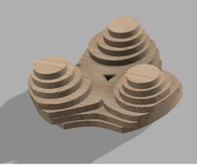
As an alternative to milling from a solid block of wood, A custom stock was created from stacking and gluing contours that were slightly larger than the final component.
