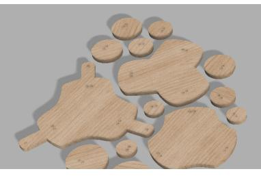
Cutting contours from a sheet of plywood or from plained solid wood eliminates the need for roughing operations. Once the custom stock is glued together, only one surfacing operation is needed for each side of the component.
