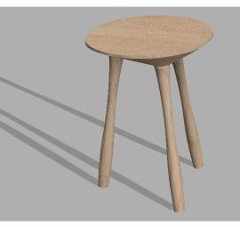
The initial concept was a CNC milled seat with three mortises for lathed dowel legs. To add stability to the stool, the legs were angled out at 80 degrees
