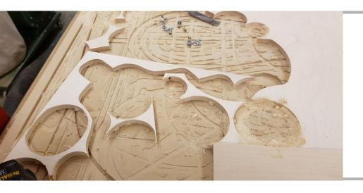
A 1/2 scale prototype of the new seat component was created from 1/2 inch Baltic birch plywood.
