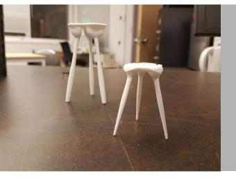
New explorations of the seat components aimed to maintain the aesthetic of a threelegged stool while increasing stability with varying leg lengths. Several 3d prints were made to test stability of new seat components and leg angles.
