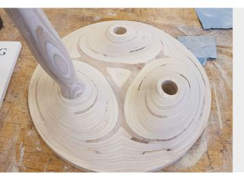
After the seat component was milled, mortises were drilled at an angle using the drill press.
