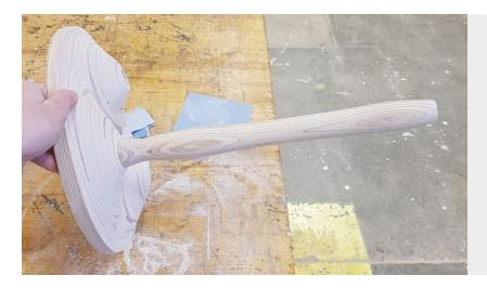
The legs were dry fitted to ensure they matched the contour of the seat component.
