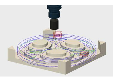
The first milling operation was a roughing pass to remove excess material.
