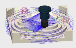
The second milling operation was a surfacing pass to that defined the contours of the seat component.
