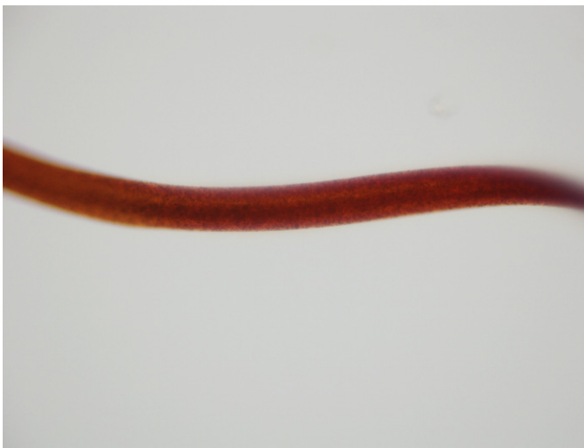
Figure 13. Viscose rayon distorted so than it resembles a trilobate fibre (mag. 400x).
