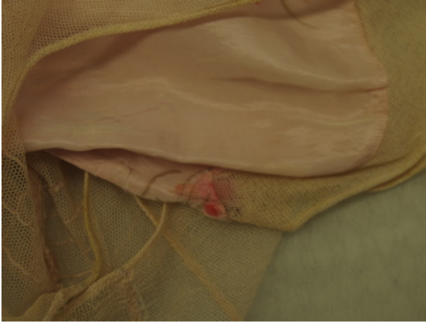
Figure 24 Transfer of pink dye from plain woven fabric to bobbinet lace in underarm region in 1930s dress (1986.31.7a)
