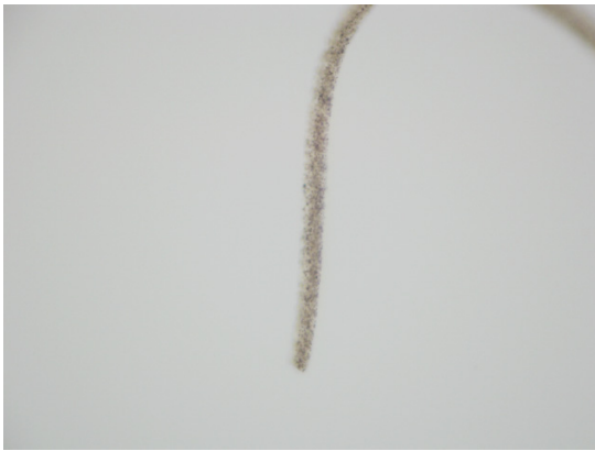
Figure 9. Fibre and mountant with similar refractive indices: Delustered acetate mounted in liquid paraffin (mag. 400x).
