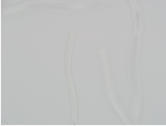
Figure 8. Fibre and mountant with similar refractive indices: Acetate mounted in liquid paraffin (mag. 400x).
