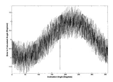
Figure A.2: Error in static angle due to quantization
