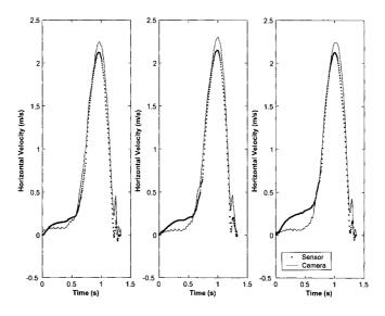
Figure 6.14: Horizontal foot velocity profiles of 3 consecutive strides - 1.1 m/s
