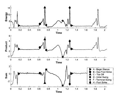
Figure 3.3: Stride detection signals derived from acceleration
