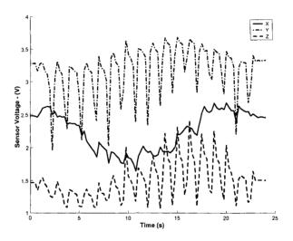
Figure 5.10: Raw AMR output for circle walk calibration
