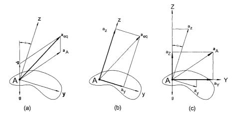
Figure 4.3: Equivalent Acceleration
