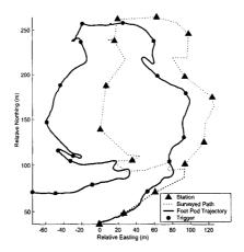
Figure 7.9: Foot pod trajectory after bias level adjustment
