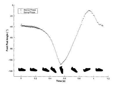
Figure 6.3: Foot pod angle profile at 1.3 m/s treadmill speed
