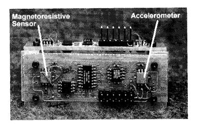
Figure 2.3: Sensor boards mounted orthogonally
