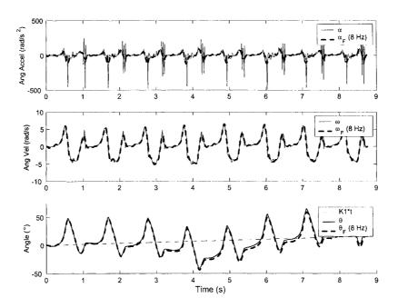
Figure 4.8: Comparison of analytical and numerical integrations of angular acceleration (top) to angular velocity (middle) and angle (bottom)
