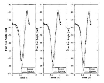
Figure 6.11: Calculated foot angle of three consecutive strides at  $1.1\,\mathrm{m/s}$
