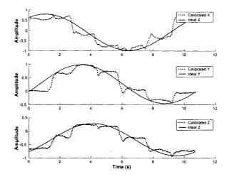
Figure 5.9: Spin calibration: Horizontal alignment corrected
