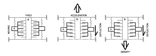
Figure 2.2: Simplified acclerometer mode of operation
