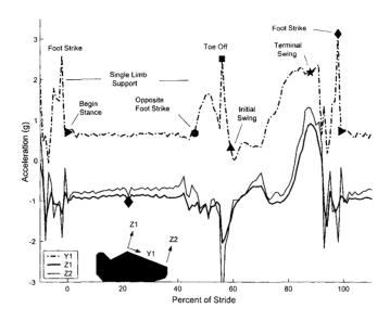
Figure 3.2: Acceleration Signals and Events
