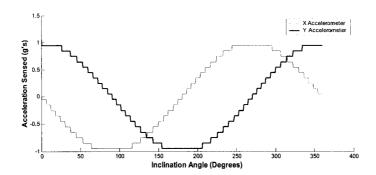
Figure A.1: Quantization of accelerometer signal
