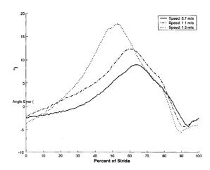
Figure 6.13: Error in dynamic foot angle profile
