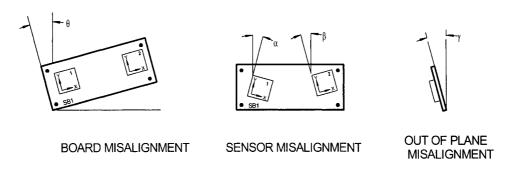
Figure B.2: Accelerometer Misalignment
