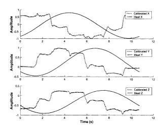
Figure 5.8: Spin calibration: Sensor output matched to ideal signal
