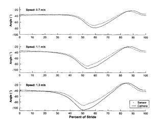
Figure 6.12: Averaged foot pod angle profiles for camera and sensors at varying speeds
