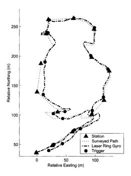
Figure 7.4: Trajectory using torso mounted ring laser gyros and constant steplength
