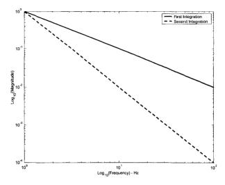
Figure 4.7: Frequency response of single and double integration
