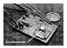
Figure 2.1: ADXL Series accelerometer on prototype board
