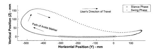
Figure 6.2: Ankle trajectory at 1.3 m/s treadmill speed
