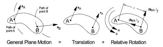
Figure 4.2: Components of General Plane Motion
