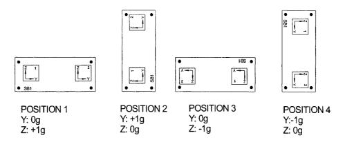
Figure B.1: Block Calibration Positions
