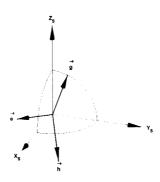
Figure 5.4: Magnetic East  $\vec{e}$  is perpendicular to both gravity  $\vec{g}$ , and magnetic field  $\vec{h}$ .
