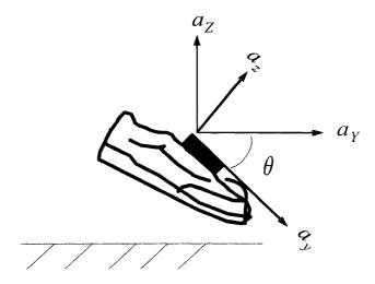
Figure 4.5: Resolving acceleration into vertical and horizontal components using foot angle.
