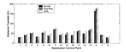
Figure 7.11: Comparison of distance measurements after bias adjustment
