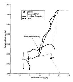
Figure 7.15: Comparison of GPS and foot pod trajectories during stationary period
