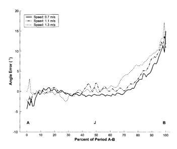
Figure 6.10: Error of static foot angle calculation
