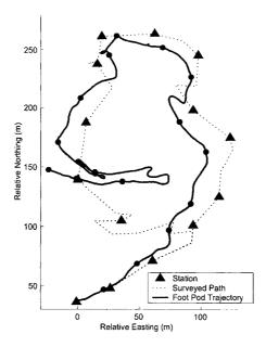
Figure 7.5: Trajectory using shoe mounted sensors
