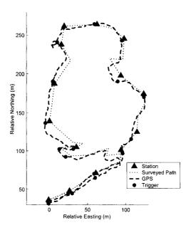
Figure 7.3: Trajectory measured by high sensitivity GPS
