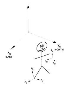
Figure 5.1: Relationship of global, user and sensor reference frames
