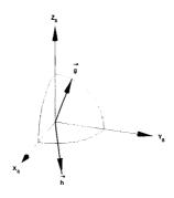
Figure 5.3: Gravitational and magnetic field vectors in the sensor frame
