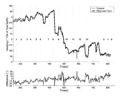
Figure 7.8: Comparison of ring laser gyro and foot pod heading
