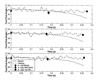
Figure 6.9: Stance phase foot angle profile for three consecutive strides
