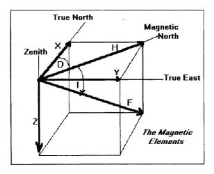
Figure C.1: Magnetic field elements, adapted from [35]
