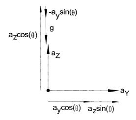
Figure 4.4: Components of horizontal and vertical acceleration
