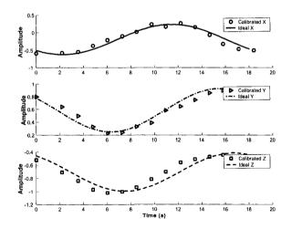
Figure 5.12: Calibrated magneto-resistive sensor signals for circle walk
