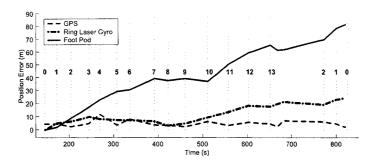
Figure 7.10: Error in position, after bias level adjustment
