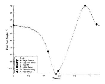
Figure 6.7: Detected gait events plotted on foot pod angle profile.
