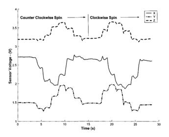
Figure 5.7: AMR sensor signals for stationary spin
