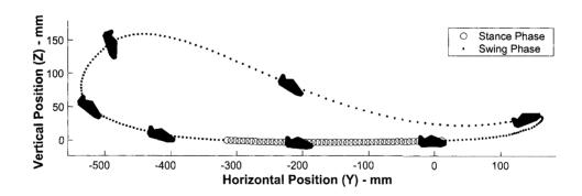
Figure 6.4: Ankle marker trajectory with foot pod angle
