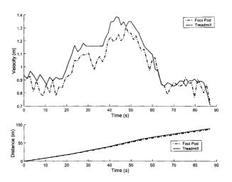
Figure 6.20: Stride velocity and distance measurement comparison
