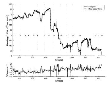
Figure 7.12: Comparison of ring laser gyro and foot pod heading after bias adjustment
