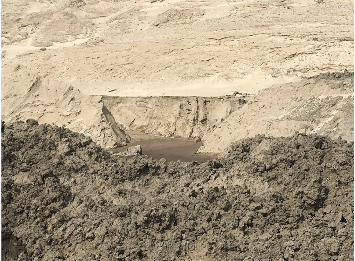
Summer Photo (f), Table 7. Washout cut (width ~1.5 m) filled with water, similar to what normally happens with pipeline leaks. Steep slope face seen behind water erosion feature.
