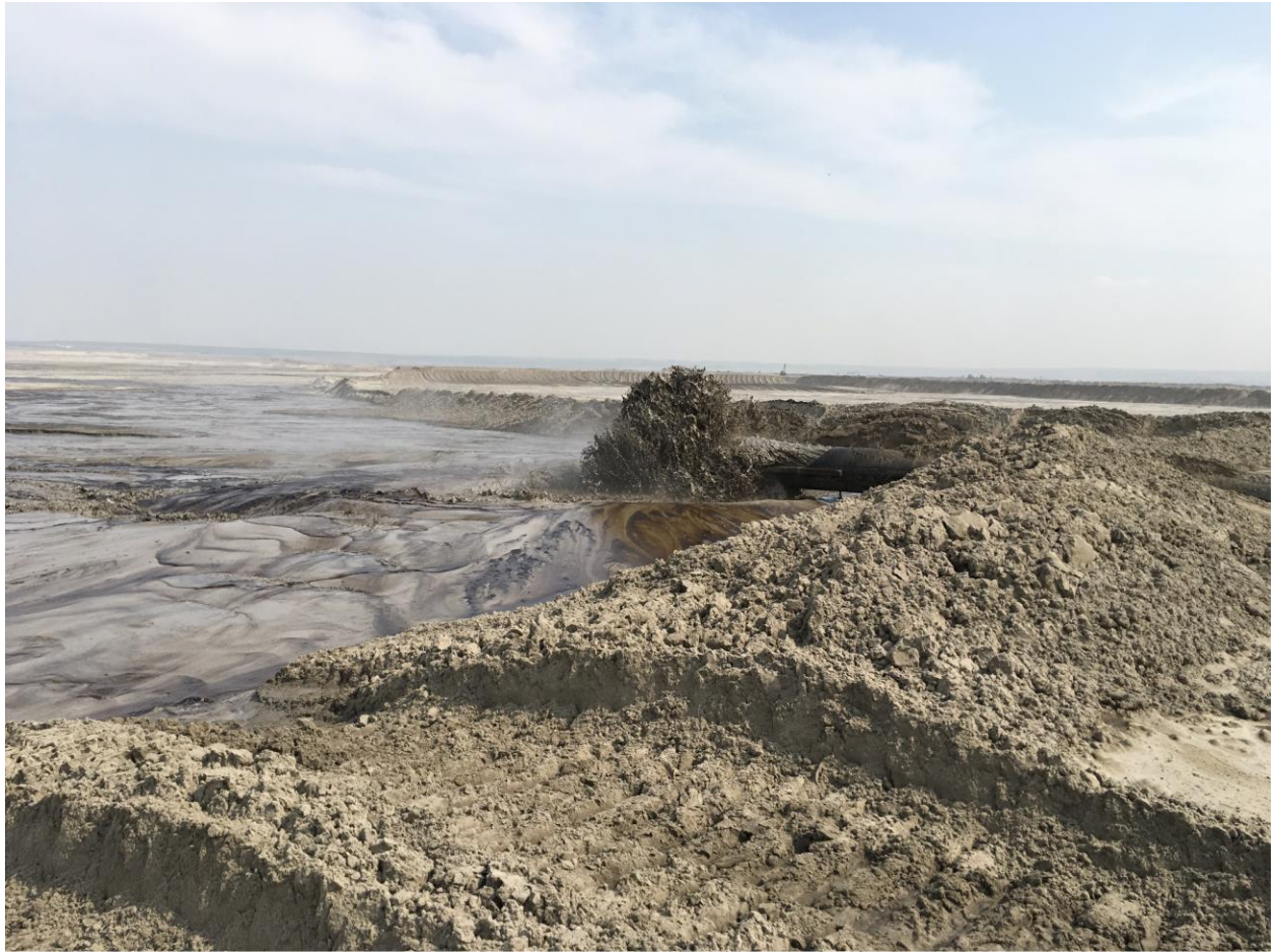
Summer Photo (c), Table 7. View of tailings discharge area and spigot.
