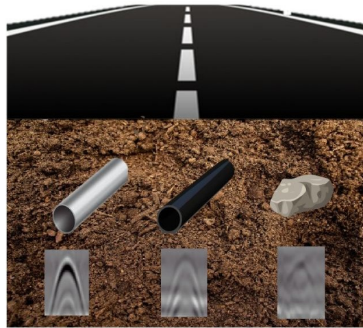
Figure 2-1: GPR signal response showing the similarity of GPR reflections for objects of different materials
