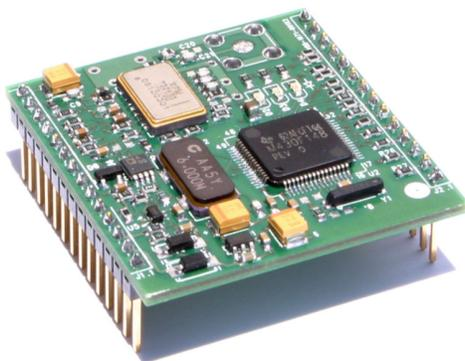
Figure 2.6: An RF Monolithics DM2200 wireless node.
