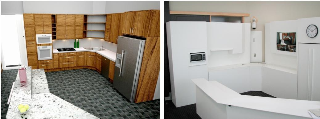
Figure 2.2: A rendering of the kitchen (left) and corresponding foam core models placed within the Smart Condo (right). Foam core consists of polystyrene foam (like foam drinking cups) sandwiched between pieces of thin cardboard.
