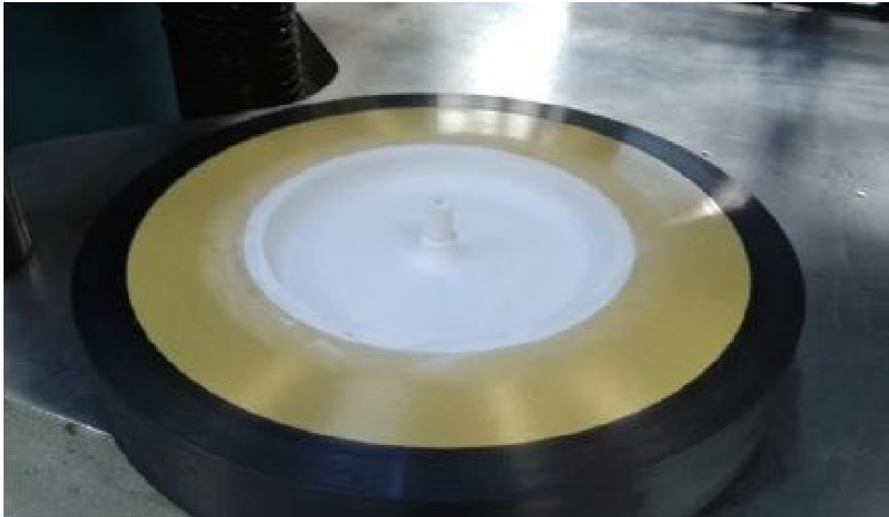
Figure 2.3: Thermal press-fit accomplished by cooling the aluminum hub with liquid nitrogen before pressing into the composite rims.
