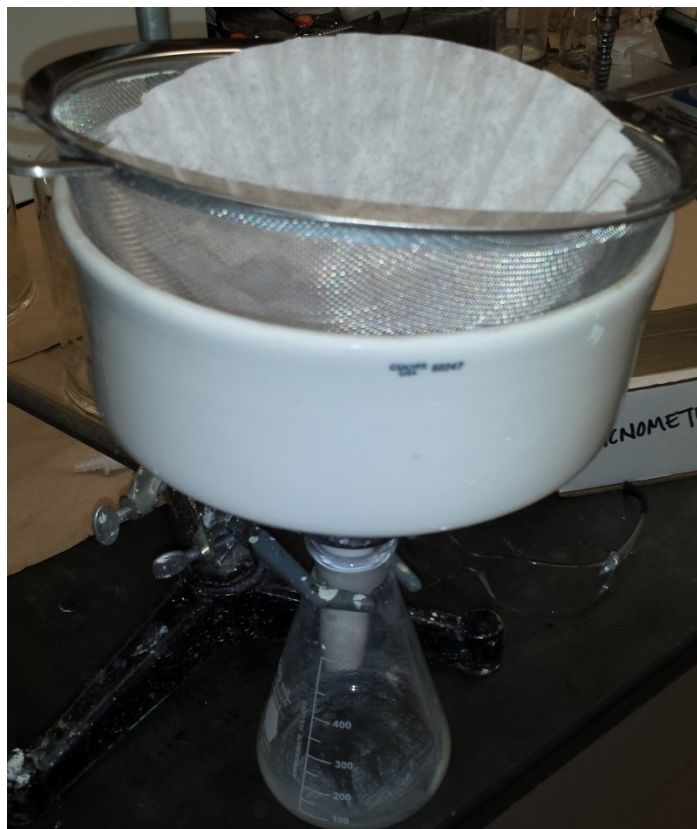
Figure 3.6: Filter paper in 1mm stainless steel within a large Buchner funnel used for paste densification
