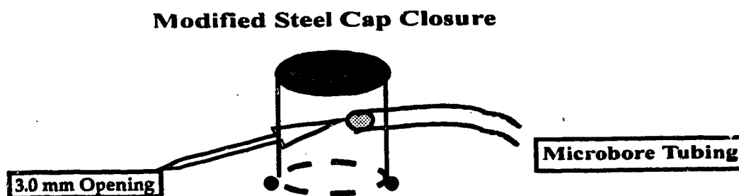
Figure 2- 4. Modified steel cap closure with 1 cm opening into which surgical microbore tubing is inserted.
